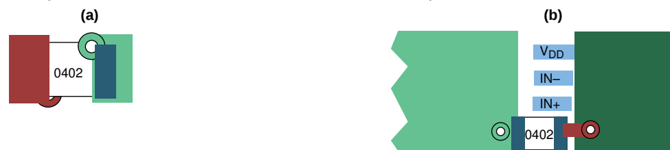
图 28. Typical Decoupling Capacitor Layouts
