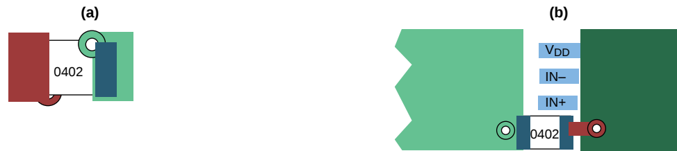
图 29. Typical Decoupling Capacitor Layouts
