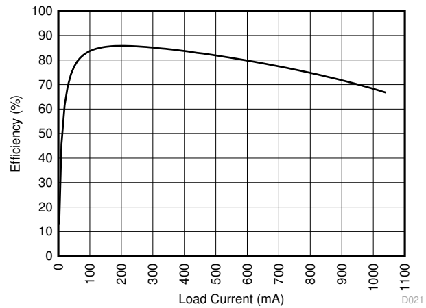
图 6-24. Efficiency vs Load Current
