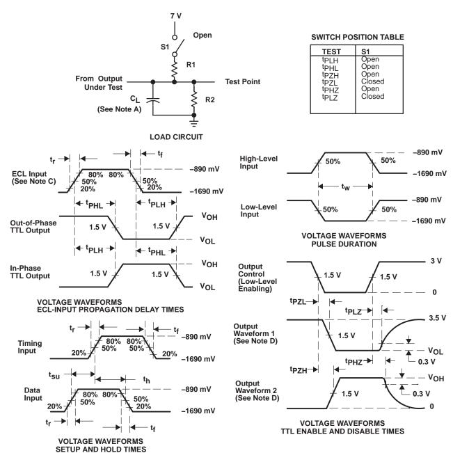
NOTES: A.C<sub>I</sub> includes probe and jig capacitance.
