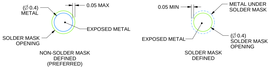
SOLDER MASK DETAILS NOT TO SCALE
