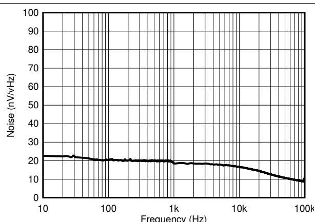
图 7-20. Noise Performance 10 Hz to 100 kHz
