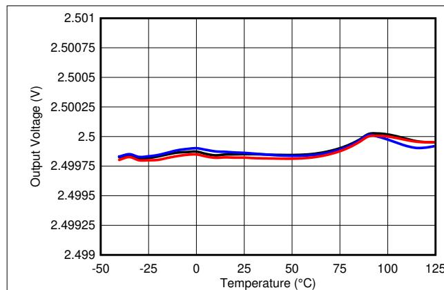
图 7-1. Output Voltage Vs Free-Air Temperature (REF7025QFKHR)
