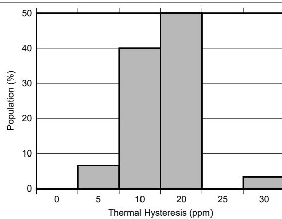
图 7-23. REF7012QFKHR Thermal Hysteresis Distribution (0°C to 70°C)
