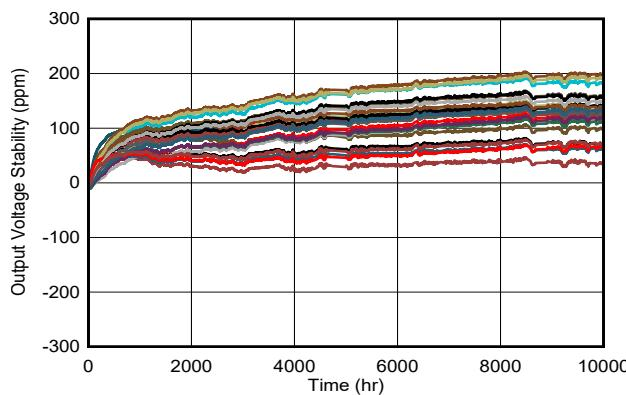
**图 8-5. Long Term Stability VSSOP -10000 hours ( $V_{OUT}$ )**
