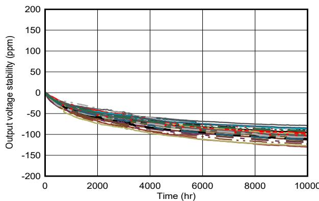
**图 8-4. Long Term Stability LCCC -10000 hours ( $V_{OUT}$ )**
