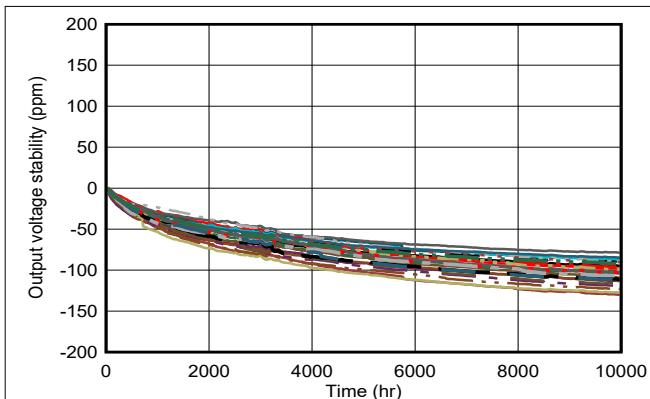
图 7-25. Long-Term Stability LCCC package (First 10000 Hours)
