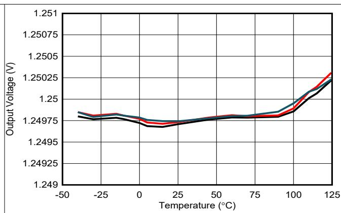
图 7-2. Output Voltage Vs Free-Air Temperature (REF7012QDGKR)
