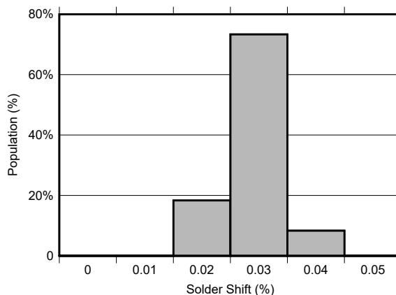
**图 8-2. Solder Shift (LCCC Package)**
