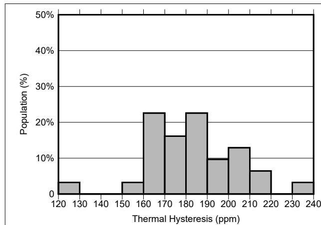
图 8-6. REF7025QFKHR Thermal Hysteresis Distribution (-40°C to 125°C)
