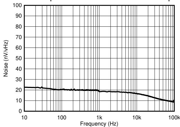
图 8-13. Noise Performance 10 Hz to 100 kHz
