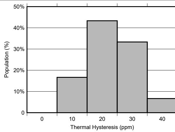
图 8-8. REF7012QFKHR Thermal Hysteresis Distribution (-40°C to 125°C)
