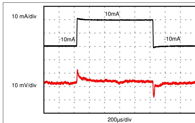
图 7-13. Load Transient Response ( $C_L = 10 \mu\text{F}$ )
