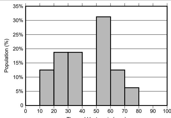
图 7-22. REF7025QFKHR Thermal Hysteresis Distribution (0°C to 70°C)
