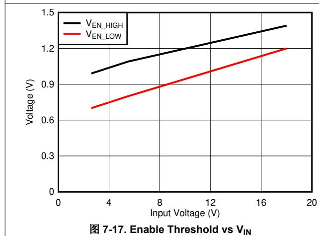
图 7-17. Enable Threshold vs  $V_{IN}$
