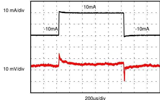
图 7-12. Load Transient Response ( $C_L = 1 \mu\text{F}$ )
