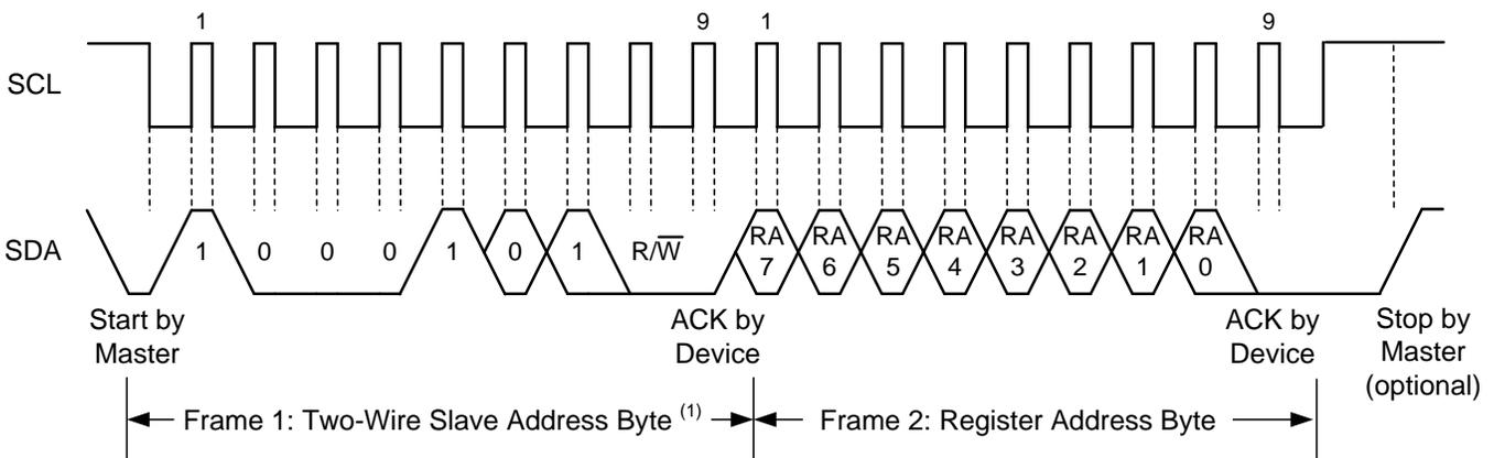
**Figure 19. Setting the I<sup>2</sup>C Register Address**
