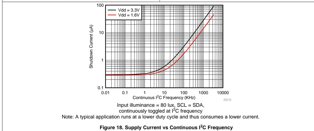
Figure 18. Supply Current vs Continuous I²C Frequency
