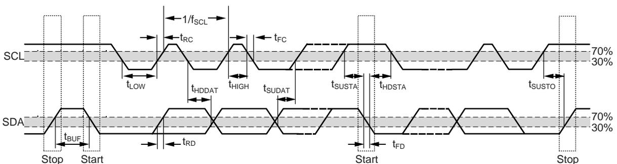
**Figure 1. I<sup>2</sup>C Detailed Timing Diagram**
