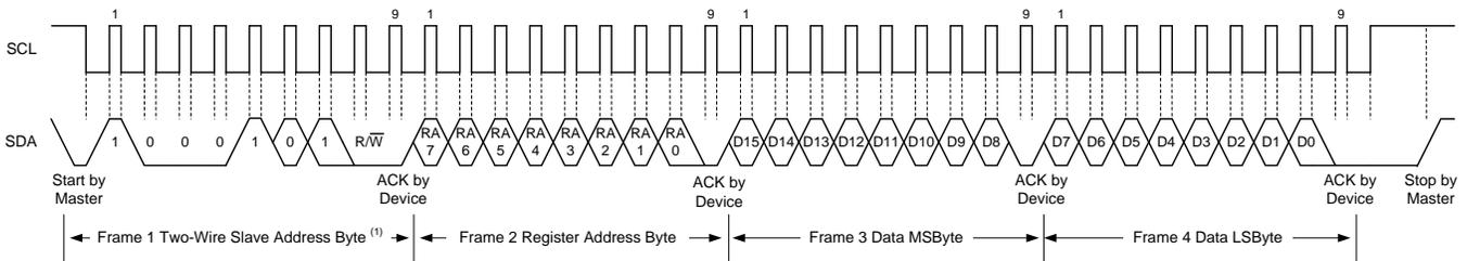
**Figure 20. I<sup>2</sup>C Write Example**
