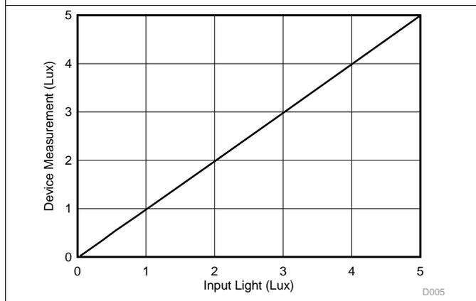
**Figure 6. Output Response vs Input Illuminance (Low Range = 0 Lux to 5 Lux)**
