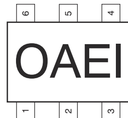
图 5-2. DBV Package, 6-Pin SOT-23 (Top View)
