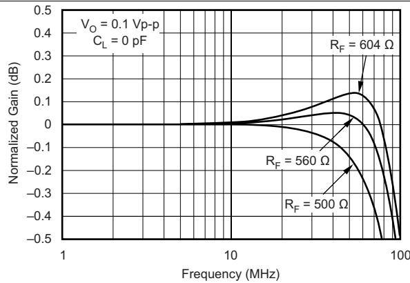
**Figure 5. 0.1-dB Gain Flatness for Various  $R_F$**
