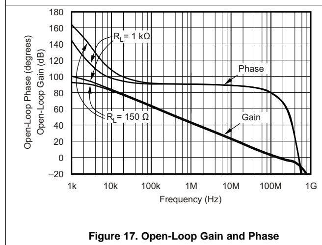
Figure 17. Open-Loop Gain and Phase
