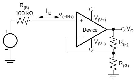
**Figure 32. Noise as a Result of  $I_{(BIAS)}$**
