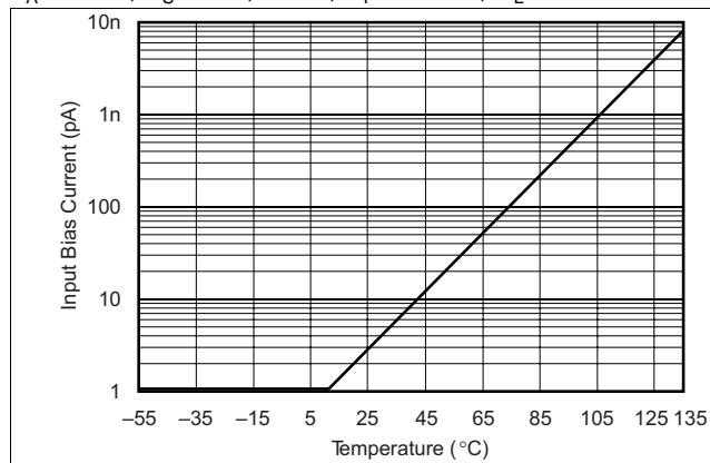
Figure 19. Input Bias Current vs Temperature
