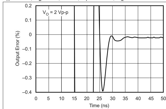
Figure 25. Output Settling Time to 0.1%
