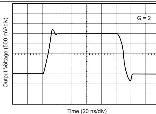
**Figure 4. Noninverting Large-Signal Step Response**
