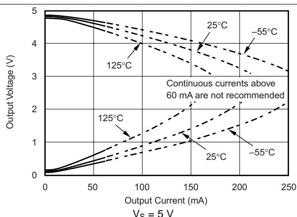
Figure 22. Output Voltage Swing vs Output Current
