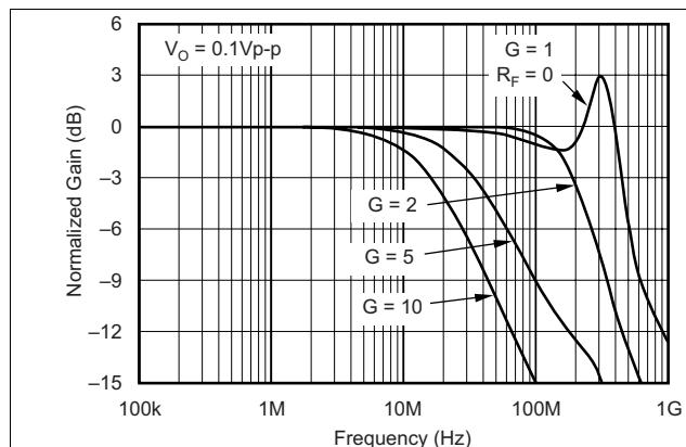
**Figure 1. Noninverting Small-Signal Frequency Response**
