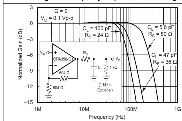
Figure 15. Frequency Response vs Capacitive Load
