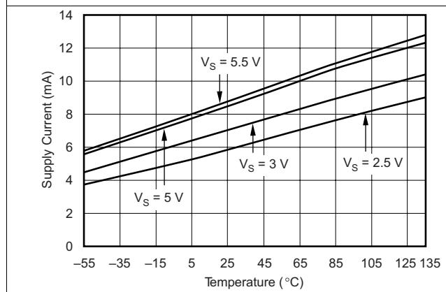
Figure 21. Supply Current vs Temperature
