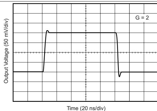
**Figure 3. Noninverting Small-Signal Step Response**
