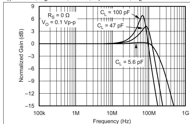
Figure 13. Frequency Response for Various  $C_L$
