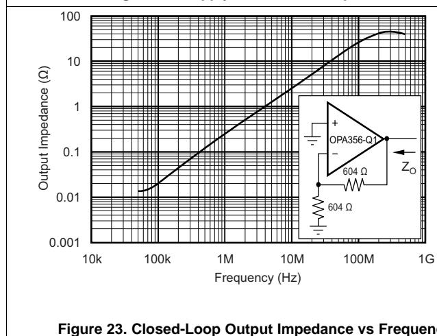
Figure 23. Closed-Loop Output Impedance vs Frequency
