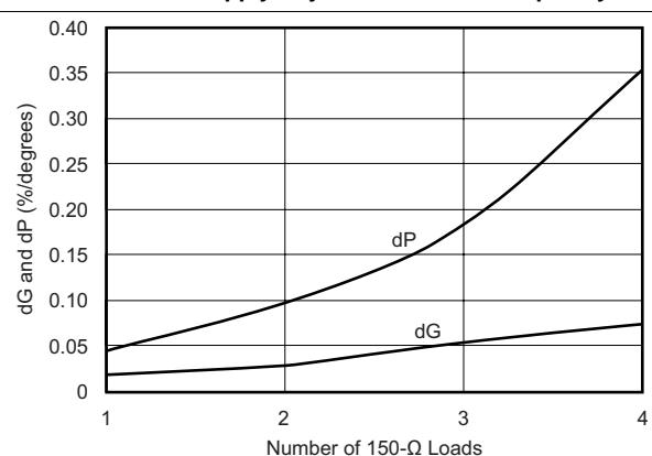
Figure 18. Composite Video Differential Gain and Phase
