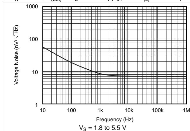
**Figure 13. Input Voltage Noise Spectral Density vs Frequency**
