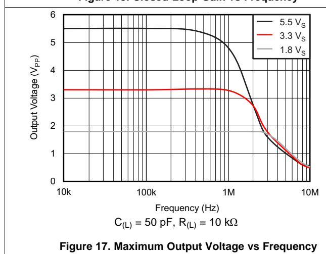
**Figure 17. Maximum Output Voltage vs Frequency**
