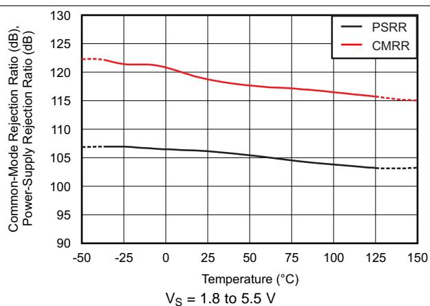
**Figure 12. CMRR and PSRR vs Temperature**
