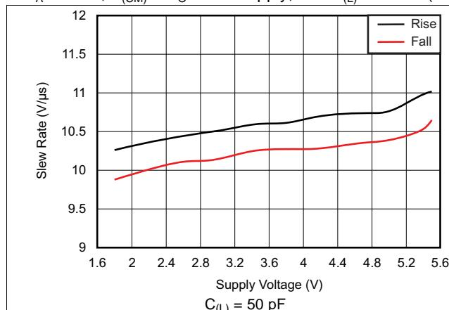
**Figure 25. Slew Rate vs Supply Voltage**
