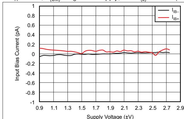
**Figure 7. Input Bias Current vs Supply Voltage**
