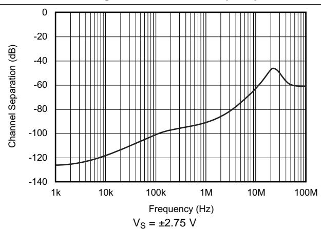
**Figure 24. Channel Separation vs Frequency**
