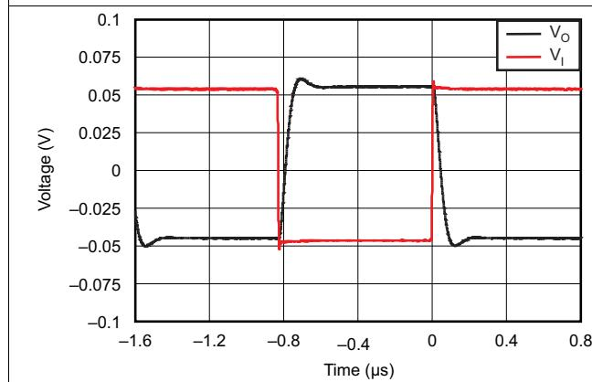
**Figure 27. Small-Signal Step Response**
