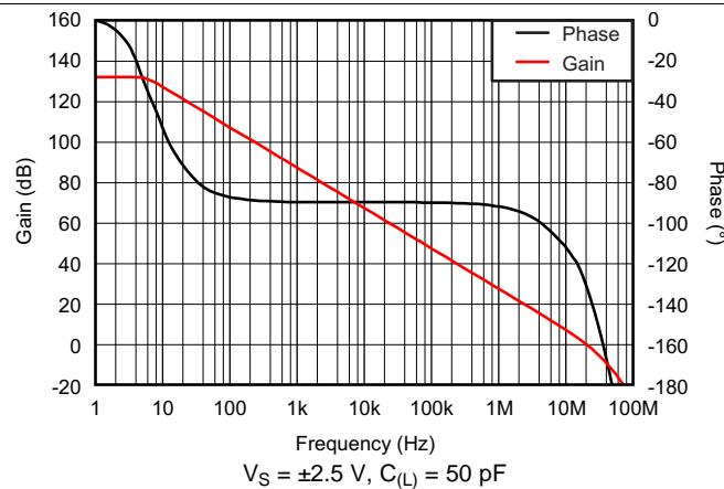
Figure 4. Open-Loop Gain and Phase vs Frequency
