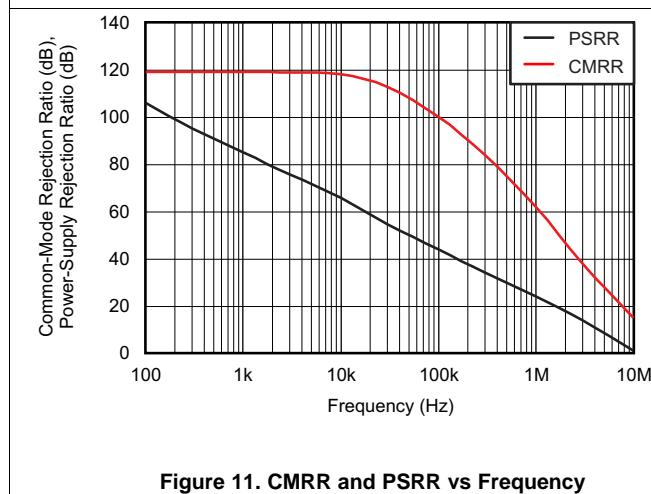
**Figure 11. CMRR and PSRR vs Frequency**
