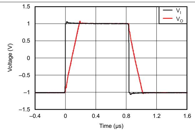
**Figure 28. Large-Signal Step Response vs Time**
