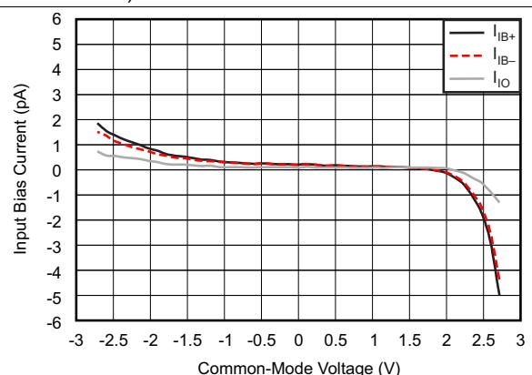
**Figure 8. Input Bias Current vs Common-Mode Voltage**
