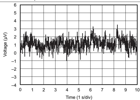
**Figure 14. 0.1-Hz to 10-Hz Input Voltage Noise**
