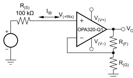
**Figure 40. Noise as a Result of  $I_{(BIAS)}$**
