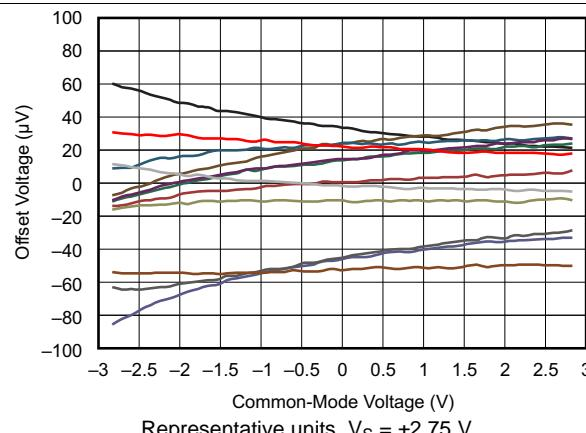
Figure 3. Offset Voltage vs Common-Mode Voltage
