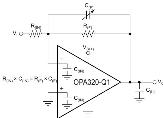
NOTE: Where  $C_{(IN)}$  is equal to the OPAX320-Q1 input capacitance (approximately 9 pF) plus any parasitic layout capacitance.
