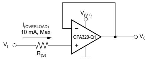
**Figure 29. Input Current Protection**
