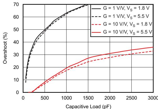
**Figure 32. Small-Signal Overshoot versus Capacitive Load (100-mV<sub>PP</sub> Output Step)**
