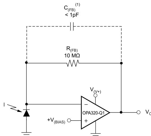
(1)  $C_{(FB)}$  is optional to prevent gain peaking.  $C_{(FB)}$  includes the stray capacitance of  $R_{(FB)}$ .
