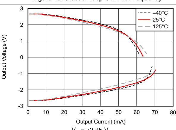
**Figure 18. Output Voltage Swing vs Output Current**
