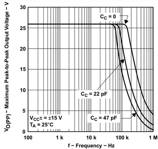
Figure 2. Maximum Peak-to-Peak Output Voltage vs Frequency
