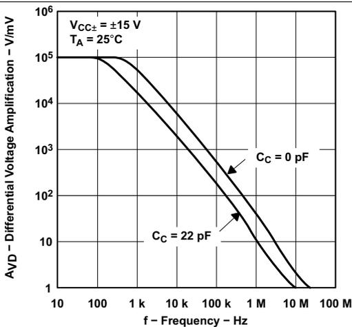
Figure 3. Large-Signal Differential Voltage Amplification vs Frequency
