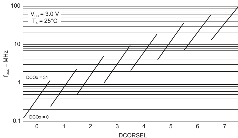
Figure 5-2. Typical DCO Frequency
