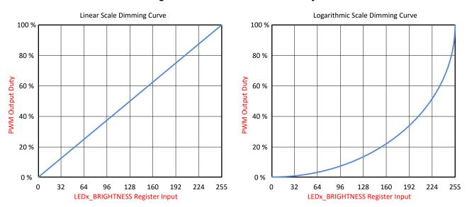
图 7-3. Logarithmic vs Linear Dimming Curve
