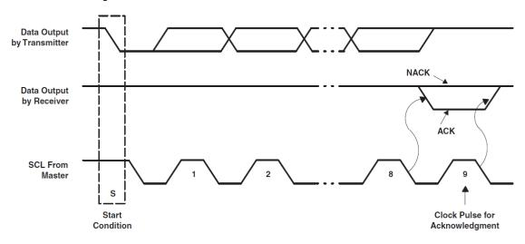
图 7-10. Acknowledge and Not Acknowledge on I<sup>2</sup>C Bus
