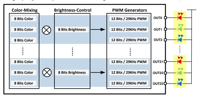
图 7-1. PWM Control Scheme for Each Channel
