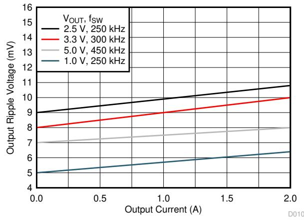
图 6-7. Voltage Ripple vs Output Current
