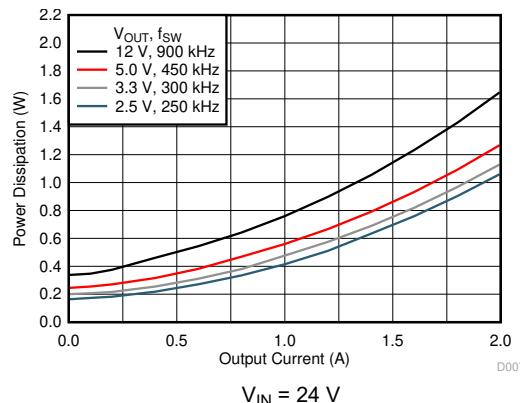
图 6-10. Power Dissipation vs Output Current
