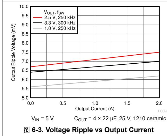
$V_{IN} = 5$  V       $C_{OUT} = 4 \times 22 \mu F, 25 V, 1210$  ceramic
