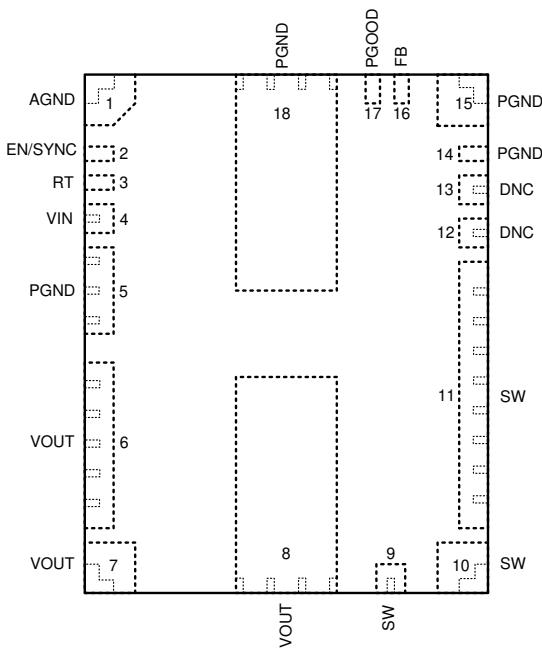
图 5-1. RLR Package 18-Pin QFN Top View
