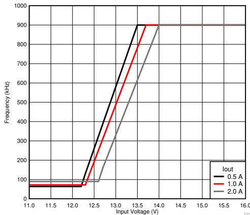
$V_{OUT} = 12 \text{ V}$
