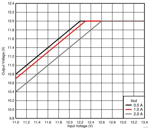
$V_{OUT} = 12 \text{ V}$
