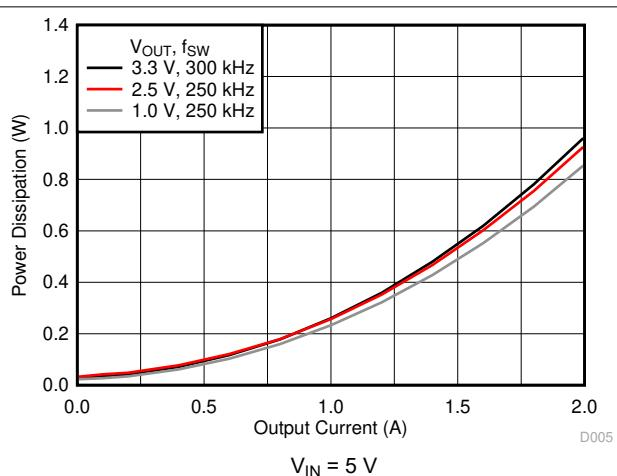
图 6-2. Power Dissipation vs Output Current
