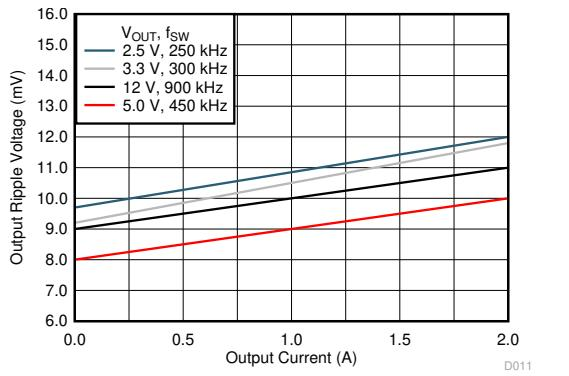
图 6-11. Voltage Ripple vs Output Current
