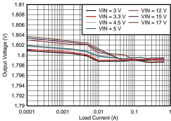
**Figure 42. Line and Load Regulation V<sub>OUT</sub> = 1.8 V**
