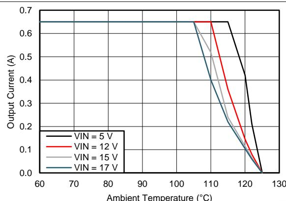
**Figure 67. Thermal Derating for θ<sub>JA</sub> = 47°C/W, V<sub>OUT</sub> = 3.3 V**
