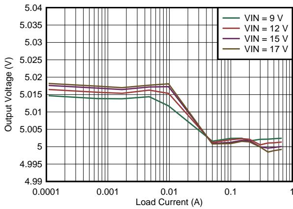
**Figure 78. Line and Load Regulation  $V_{OUT} = 5.0$  V**
