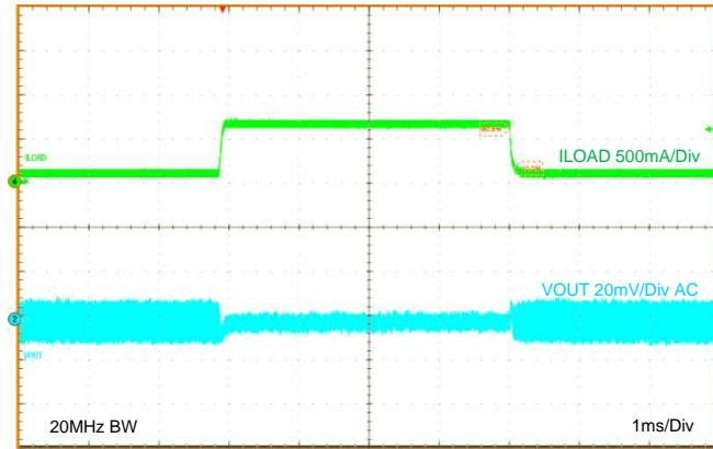
**Figure 72. Load Transient  $V_{OUT} = 5.0 \text{ V}$**
