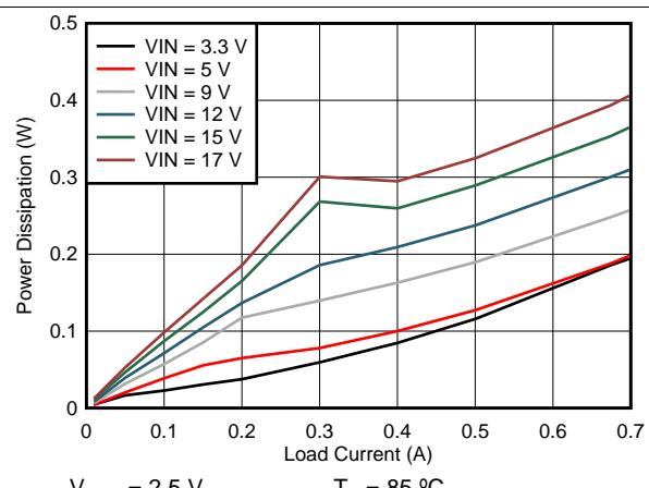
Figure 5. Power Dissipation
