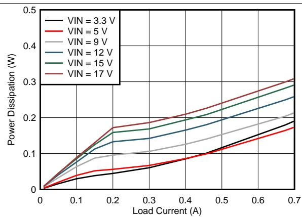
Figure 3. Power Dissipation
