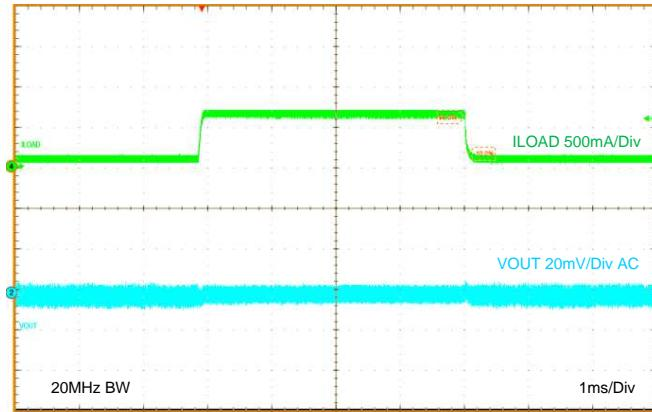
Figure 36. Load Transient  $V_{OUT} = 1.8 \text{ V}$
