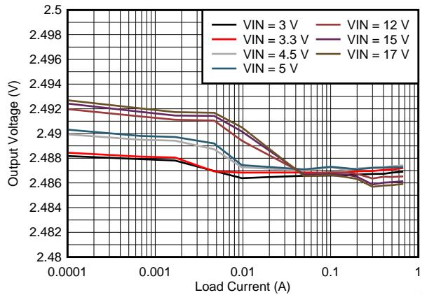
**Figure 54. Line and Load Regulation  $V_{OUT} = 2.5\text{ V}$**
