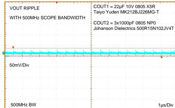
**Figure 51. 500MHz Oscilloscope Bandwidth, 3x1000pF
