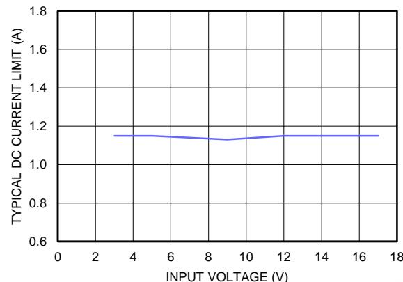
**Figure 41. Typical Current Limit V<sub>OUT</sub> = 1.8 V, T<sub>A</sub> = 85 °C**
