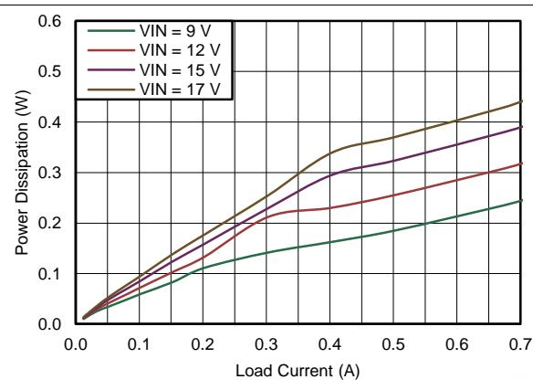
**Figure 71. Power Dissipation  $V_{OUT} = 5.0 \text{ V}$**
