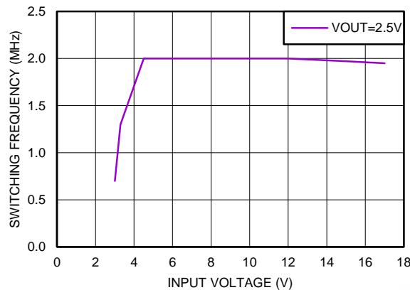
**Figure 52. Typical Switching Frequency at 650mA Load
