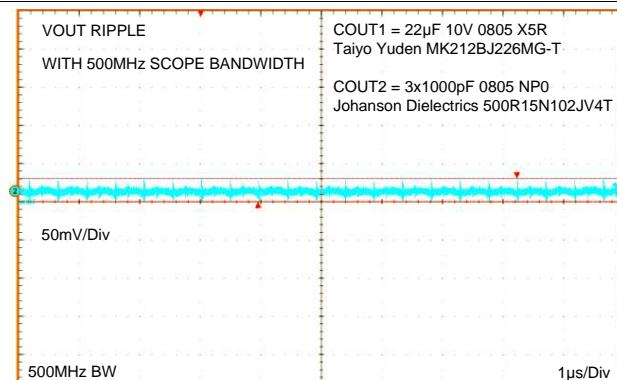
**Figure 75. 500 MHz Oscilloscope Bandwidth, 3x1000 pF
