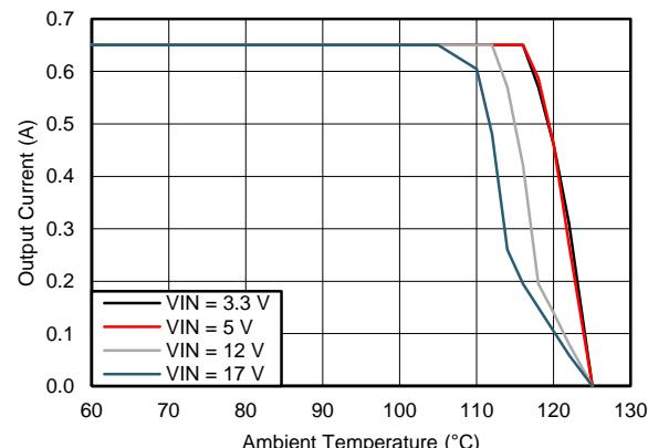
**Figure 43. Thermal Derating for θ<sub>JA</sub>=47°C/W, V<sub>OUT</sub> = 1.8 V**
