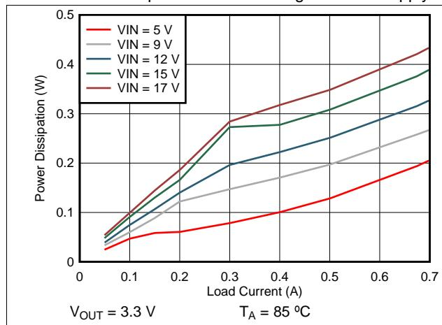
**Figure 6. Power Dissipation**
