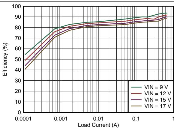
**Figure 70. Efficiency  $V_{OUT} = 5.0 \text{ V}$**
