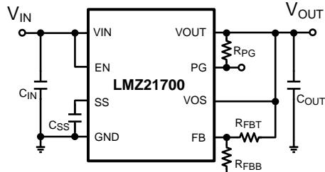
Figure 20. Typical Applications Circuit
