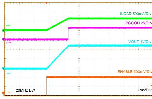
**Figure 49. Startup  $V_{OUT} = 2.5\text{ V}$**
