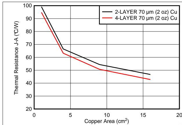
Figure 2. Package Thermal Resistance vs. Board Copper Area, No Air Flow
