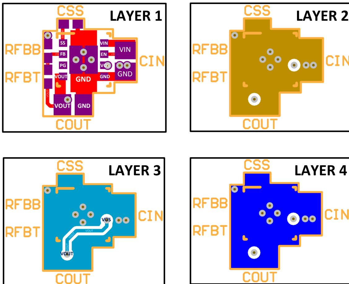
Figure 82. 35mm<sup>2</sup> Solution Size (Single Sided)
