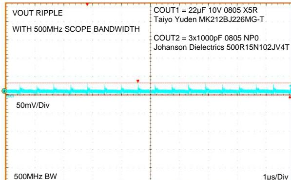
**Figure 27. 500MHz Oscilloscope Bandwidth, 3x1000pF
