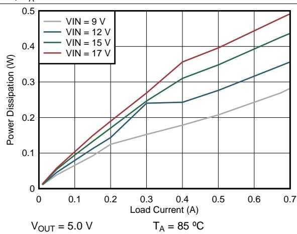
**Figure 7. Power Dissipation**
