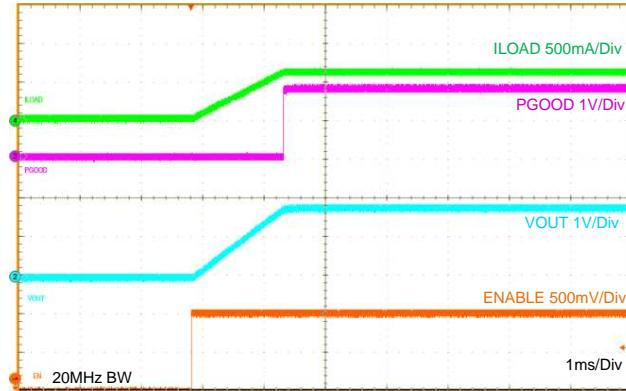
Figure 37. Startup  $V_{OUT} = 1.8 \text{ V}$
