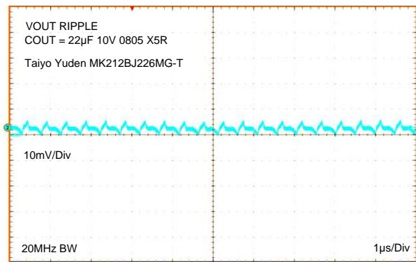
**Figure 62. 20 MHz Oscilloscope Bandwidth
