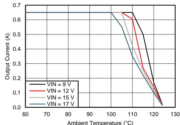
**Figure 79. Thermal Derating for  $\theta_{JA} = 47^\circ\text{C}/\text{W}$ ,  $V_{OUT} = 5.0$  V**
