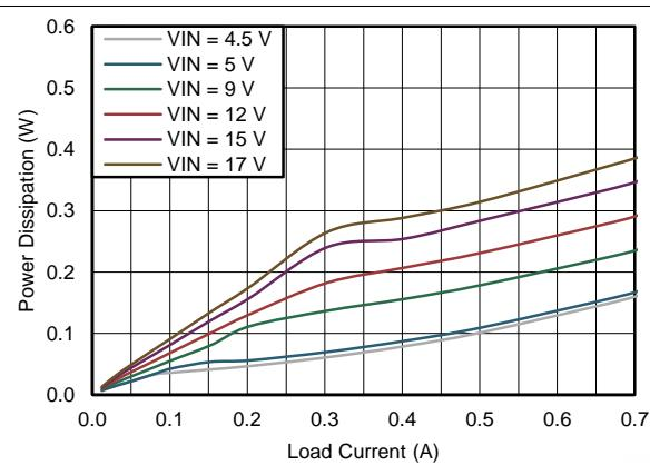
**Figure 59. Power Dissipation  $V_{OUT} = 3.3\text{ V}$**
