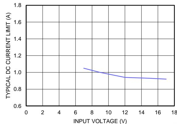
**Figure 77. Typical Current Limit  $V_{OUT} = 5.0$  V,  $T_A = 85$  °C**
