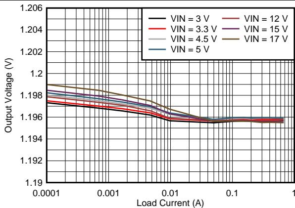
**Figure 30. Line and Load Regulation  $V_{OUT} = 1.2V$**
