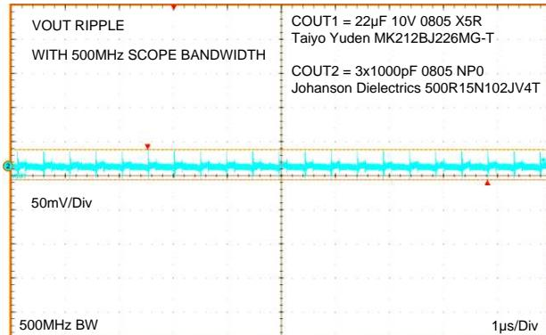
**Figure 63. 500MHz Oscilloscope Bandwidth, 3x1000 pF
