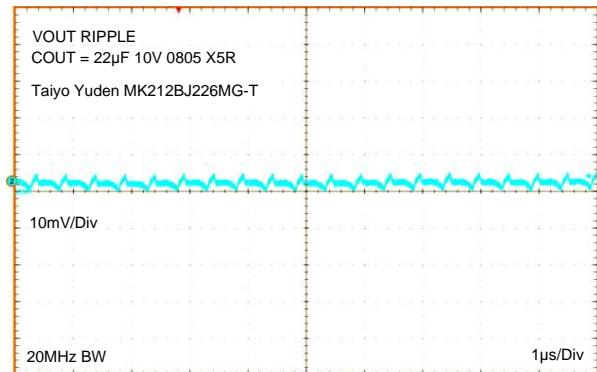
**Figure 50. 20MHz Oscilloscope Bandwidth
