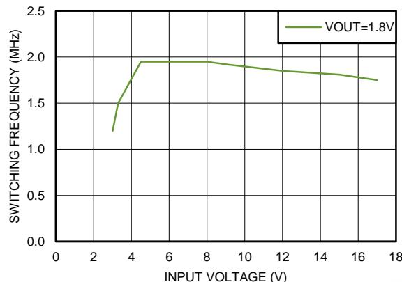
**Figure 40. Typical Switching Frequency at 650mA Load
