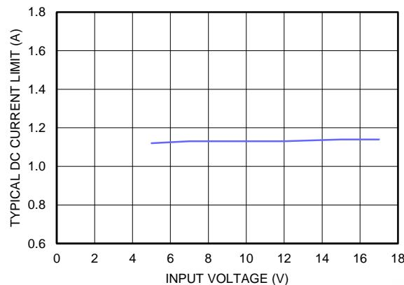
**Figure 65. Typical Current Limit V<sub>OUT</sub> = 3.3 V, T<sub>A</sub> = 85 °C**
