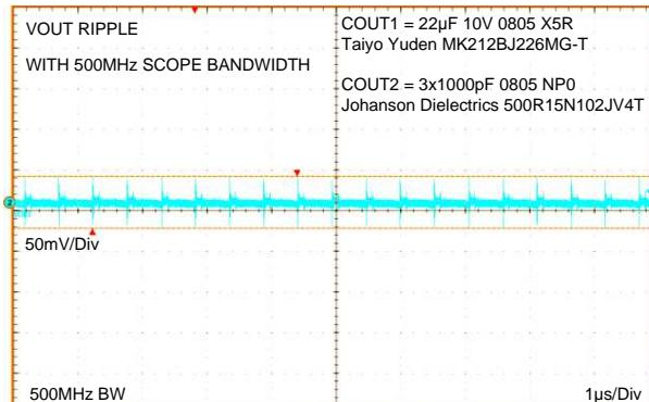
**Figure 39. 500MHz Oscilloscope Bandwidth, 3x1000pF
