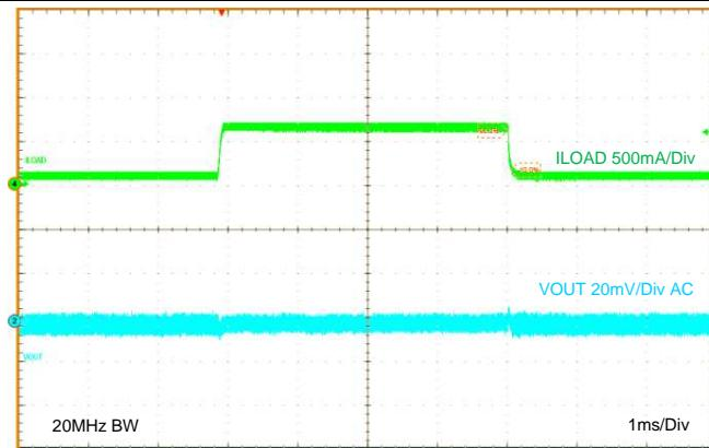
**Figure 48. Load Transient  $V_{OUT} = 2.5\text{ V}$**
