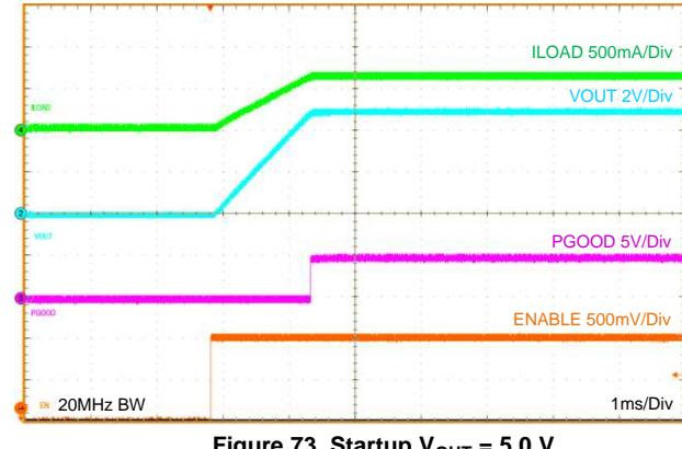
**Figure 73. Startup  $V_{OUT} = 5.0 \text{ V}$**
