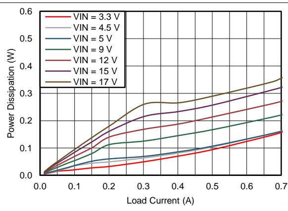
**Figure 47. Power Dissipation  $V_{OUT} = 2.5\text{ V}$**
