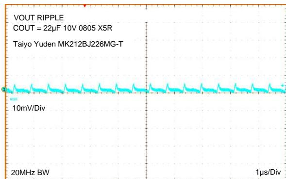
**Figure 26. 20MHz Oscilloscope Bandwidth
