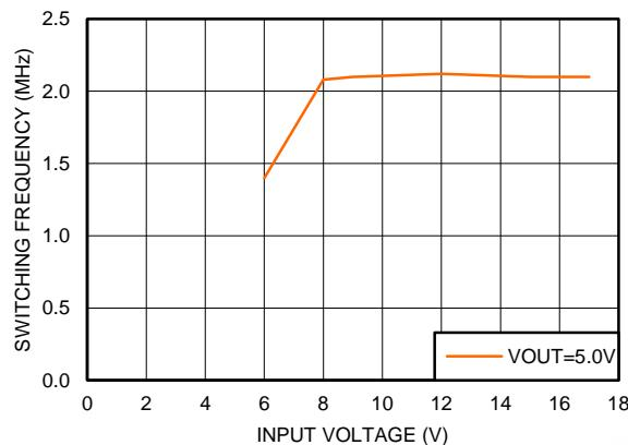
**Figure 76. Typical Switching Frequency at 650 mA Load
