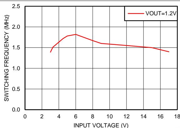
**Figure 28. Typical Switching Frequency at 650mA Load
