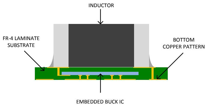
**Figure 13. LMZ21700 Package Construction Cross Section
