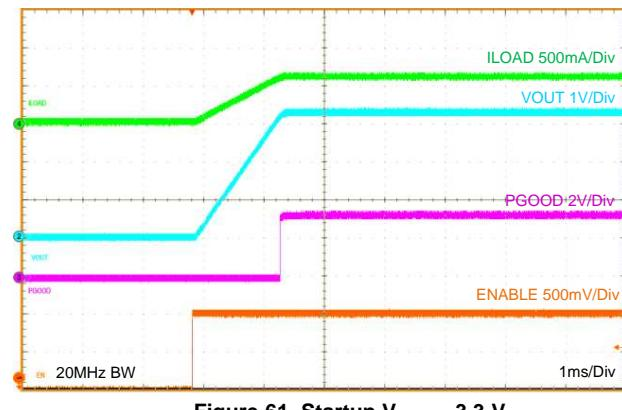
**Figure 61. Startup  $V_{OUT} = 3.3\text{ V}$**
