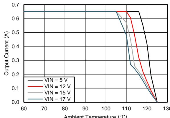
**Figure 55. Thermal Derating for  $\theta_{JA}=47\text{ }^{\circ}\text{C}/\text{W}$ ,  $V_{OUT} = 2.5\text{ V}$**
