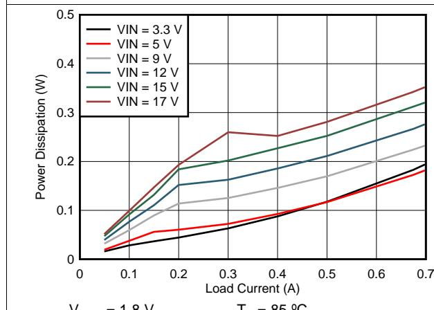
Figure 4. Power Dissipation
