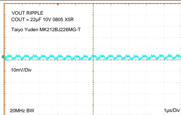
**Figure 74. 20 MHz Oscilloscope Bandwidth
