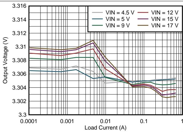
**Figure 66. Line and Load Regulation V<sub>OUT</sub> = 3.3 V**
