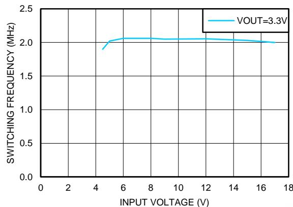
**Figure 64. Typical Switching Frequency at 650mA Load
