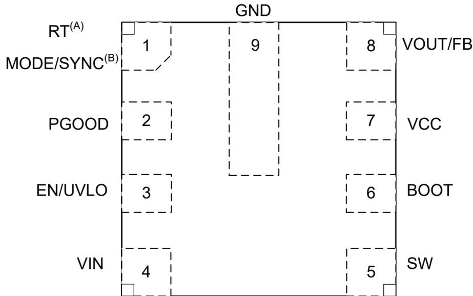
A. See [Device Comparison Table](#) for more details. Pin 1 is factory-set for externally adjustable switching frequency RT variants only.
