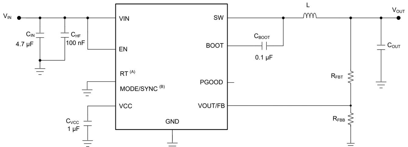
A. The RT pin is factory-set for externally adjustable switching frequency RT variants only. Tying this pin to VCC results in 1-MHz switching frequency. See [节 8.3.3](#) for details.
