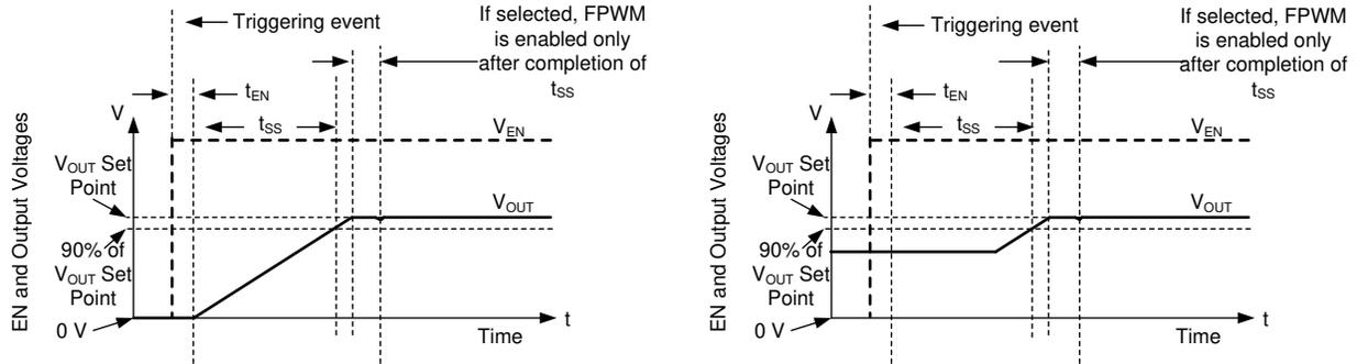
**图 8-10. Soft Start With and Without Pre-bias Voltage**
