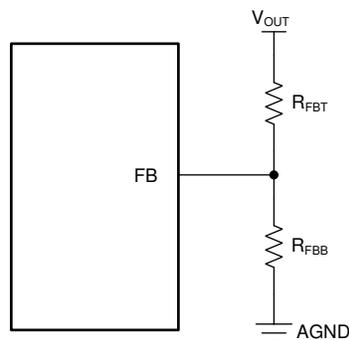
**图 8-9. Setting Output Voltage for Adjustable Output Variant**
