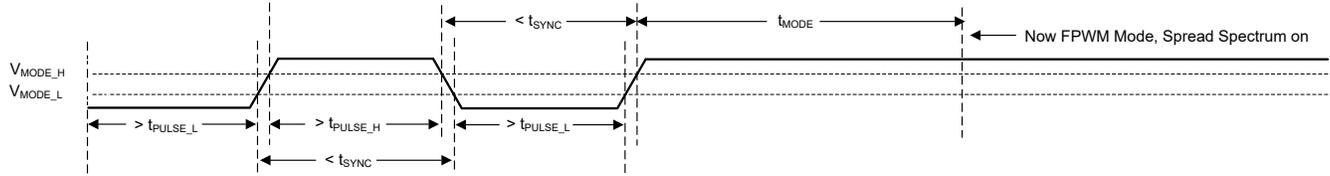
图 8-6. Transition from SYNC Mode to FPWM Mode
