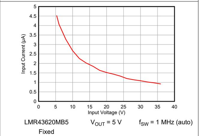
图 9-6. Input Switching Current vs Input Voltage
