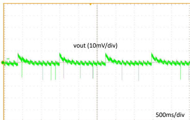
LMR43620MB5 Fixed V_{OUT} = 5\text{ V} V_{IN} = 24\text{ V} f_{SW} = 1\text{ MHz (auto)} I_{OUT} = \text{Open}
