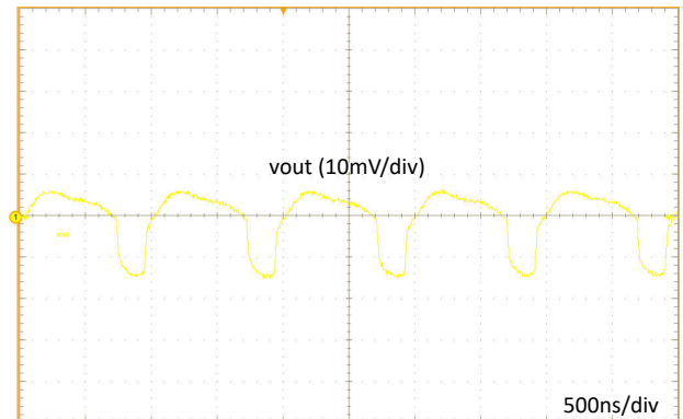
LMR43620MB5 Fixed V_{OUT} = 5\text{ V} V_{IN} = 24\text{ V} f_{SW} = 1\text{ MHz (auto)} I_{OUT} = 2\text{ A}
