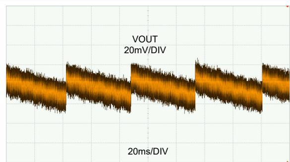
LMR43606MSC3  $V_{OUT} = 3.3V$  2.2MHz (自动)
