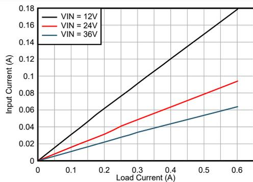
LMR43606MSC3  $V_{OUT} = 3.3V$  2.2MHz (自动)
