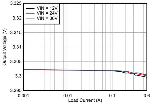
LMR43606MSC3  $V_{OUT} = 3.3V$  2.2MHz (自动)
