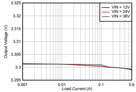
LMR43606MSC3  $V_{OUT} = 3.3V$  400kHz (自动)
