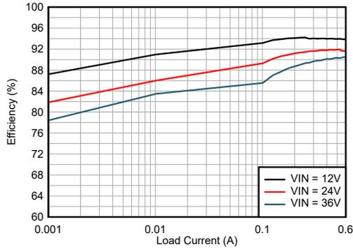
LMR43606RS5  $V_{OUT} = 5V$  400kHz (自动)
