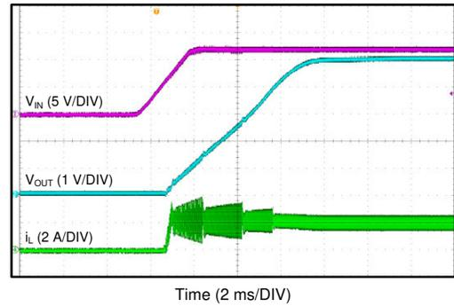
$V_{IN} = 12V$        $V_{OUT} = 5V$        $I_{OUT} = 2A$
