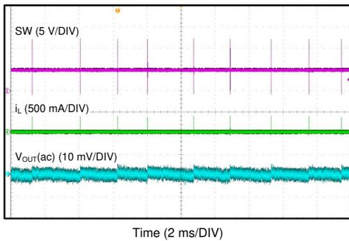
$V_{IN} = 12V$        $V_{OUT} = 5V$        $I_{OUT} = 0A$
