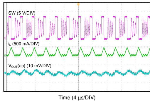
$V_{IN} = 12V$        $V_{OUT} = 5V$        $I_{OUT} = 100mA$
