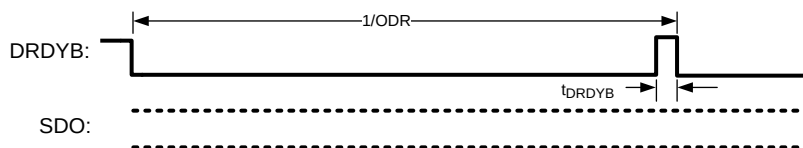
Figure 58. DRDYB Behavior for an ADC_DOUT not Read
