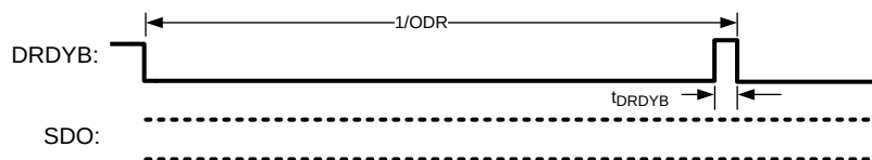
Figure 58. DRDYB Behavior for an ADC_DOUT not Read
