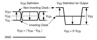
图 7-2. Two Different Definitions for Differential Output Signals
