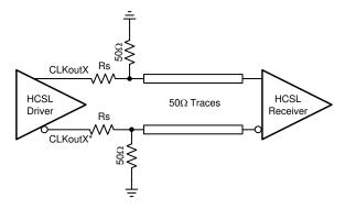
图 9-6. HCSL Operation, DC Coupling
