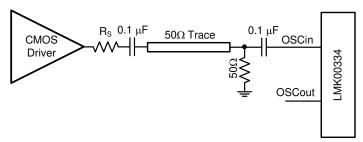
图 9-4. Driving OSCin With a Single-Ended Input
