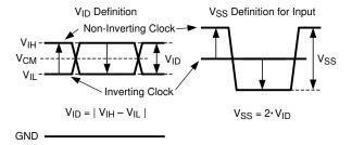
图 7-1. Two Different Definitions for Differential Input Signals
