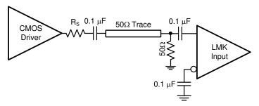
图 9-2. Single-Ended LVCMOS Input, AC Coupling
