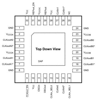
图 5-1. RTV Package 32-Pin WQFN Top View
