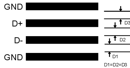
Figure 12. Ideal Diode Trace Layout
