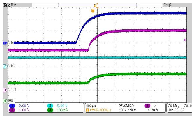
图 22. Switchover from VIN2 3.3 V to VIN1 5 V
