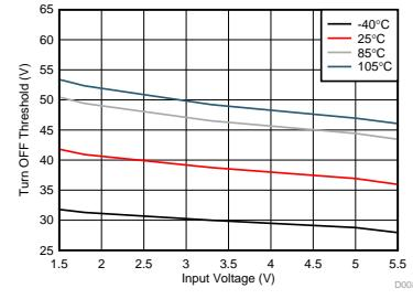
图 6. Turn OFF Threshold vs Input Voltage
