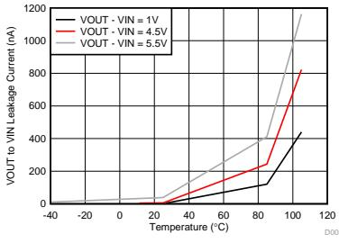
图 3. Reverse Leakage Current vs Junction Temperature
