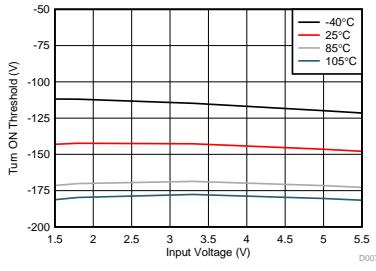
图 5. Turn ON Threshold vs Input Voltage
