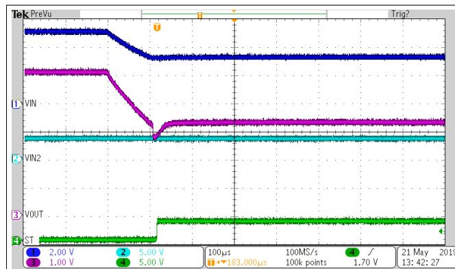
图 18. Switchover from VIN1 (5 V) to VIN2 (3.3 V)
