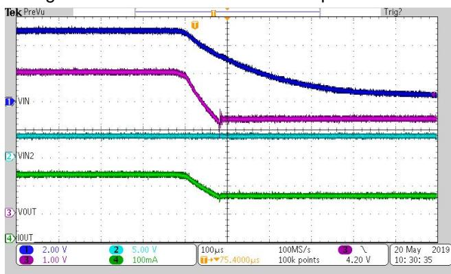
图 21. Switchover from VIN1 5 V to VIN2 3.3 V
