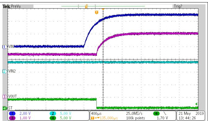
图 19. Switchover from VIN2 (3.3V) to VIN1 (5V)
