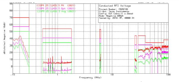
$V_{IN} = 24V$   $V_{OUT} = 5V$   $I_{OUT} = 3.5A$  | 2200kHz
