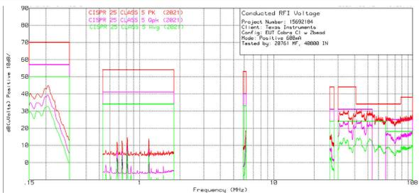
$V_{IN} = 24V$   $V_{OUT} = 5V$   $I_{OUT} = 3.5A$  | 2200kHz
