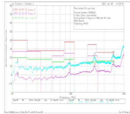
$V_{OUT} = 5\text{ V}$        $F_{SW} = 2.2\text{ MHz}$        $I_{OUT} = 4\text{ A}$
