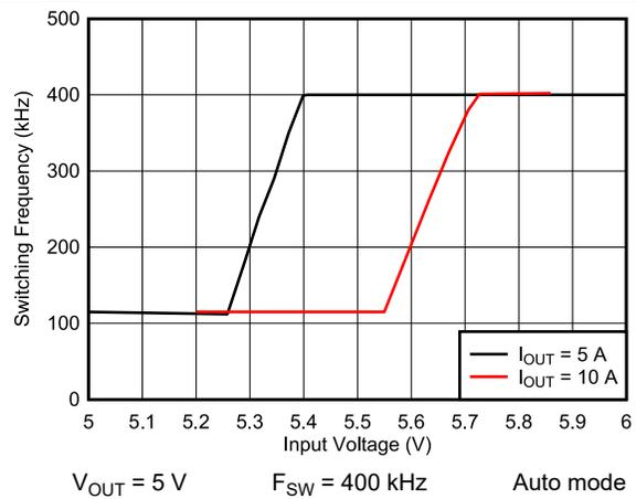
图 9-25. Frequency Dropout
