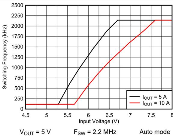
图 9-27. Frequency Dropout
