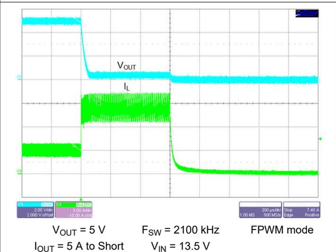
**图 9-34. Short Circuit Protection**
