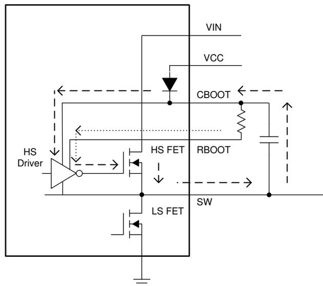
**图 8-10. Simplified Circuit Showing How RBOOT Functions**
