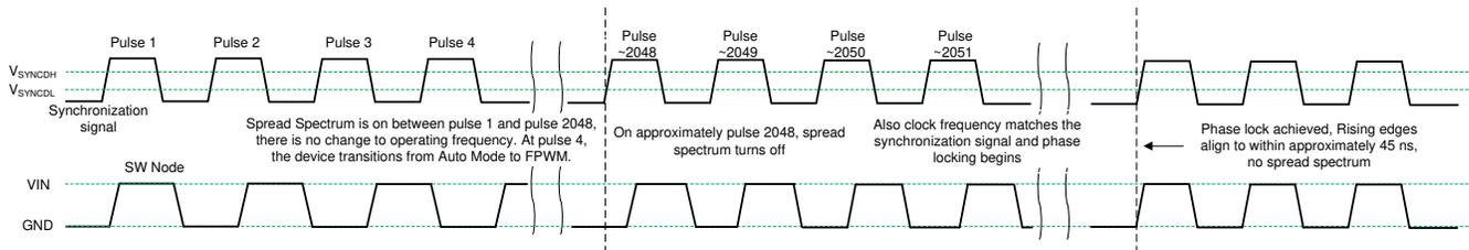
At pulse 4, the synchronization signal is detected. After approximately pulse 2048, it is ready to synchronize and the frequency is adjusted using a glitch-free technique. Later, phase is locked.
