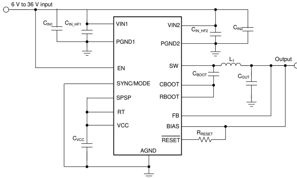
图 9-2. Example Application Circuit - 400-kHz Fixed Output
