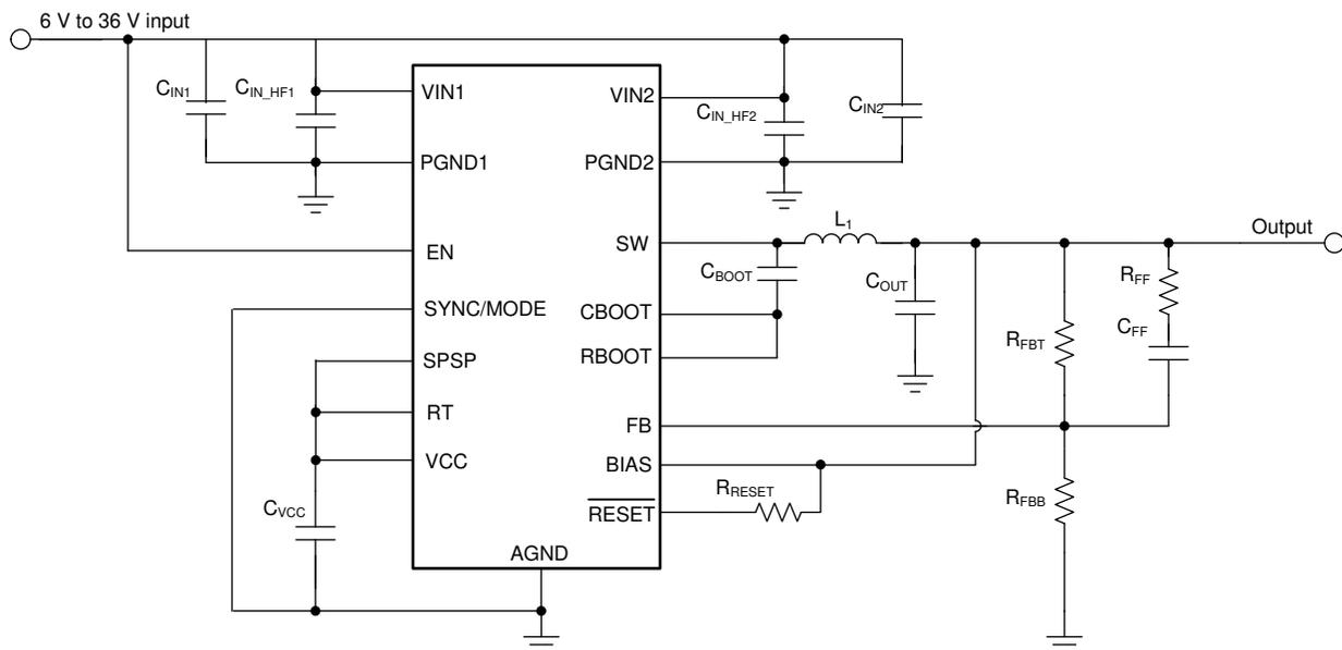
图 9-1. Example Application Circuit - 400-kHz Adjustable Output
