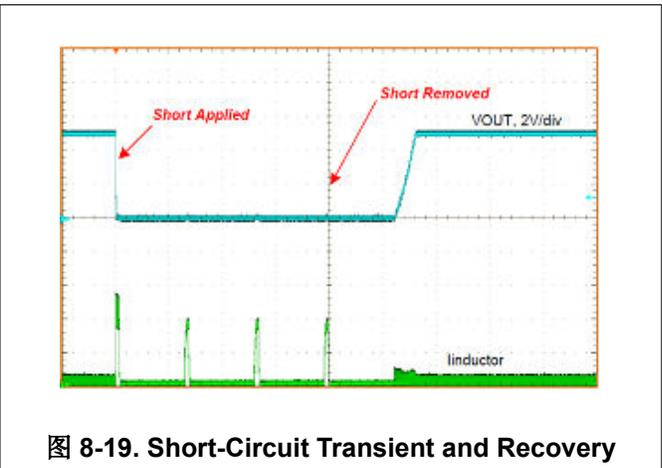
图 8-19. Short-Circuit Transient and Recovery
