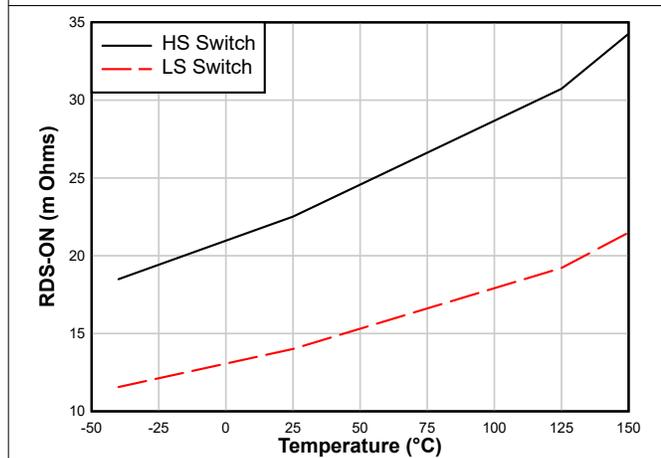
图 7-3. High-side and Low-side Switches  $R_{DS\_ON}$
