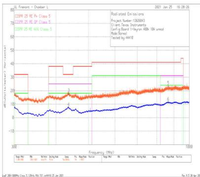
$V_{OUT} = 5\text{ V}$        $F_{SW} = 400\text{ kHz}$        $I_{OUT} = 10\text{ A}$
