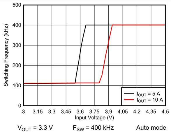
图 9-26. Frequency Dropout
