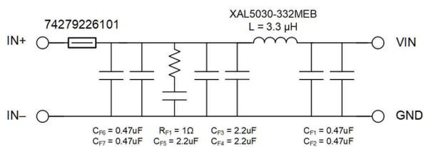
图 9-51. Recommended Input EMI Filter
