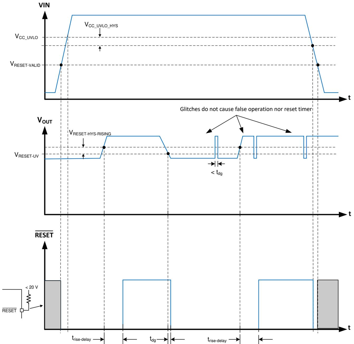
图 8-8. RESET Timing Diagram (Excludes OV Events)
