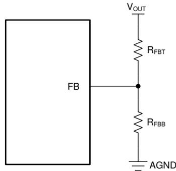
**图 8-1. Setting Output Voltage of Adjustable Versions**
