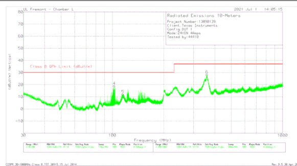
图 9-46. Radiated EMI Bicon Vertical versus CISPR11/32 Limits
