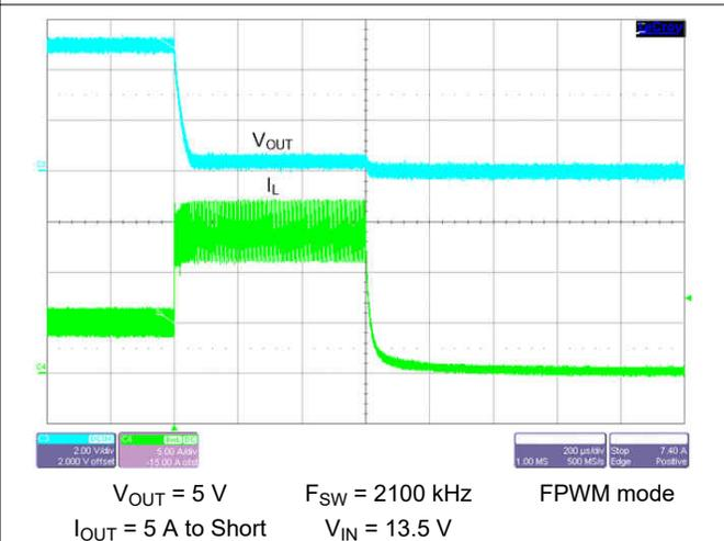
图 9-34. Short Circuit Protection
