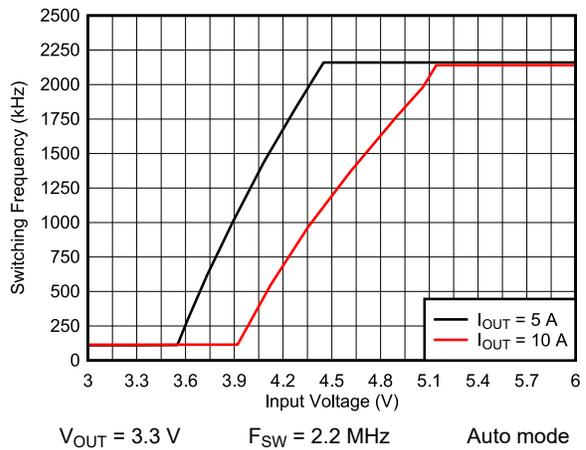
图 9-28. Frequency Dropout
