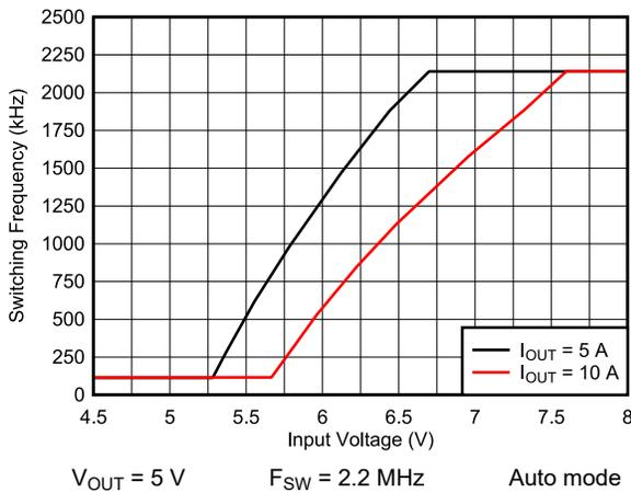
图 9-27. Frequency Dropout
