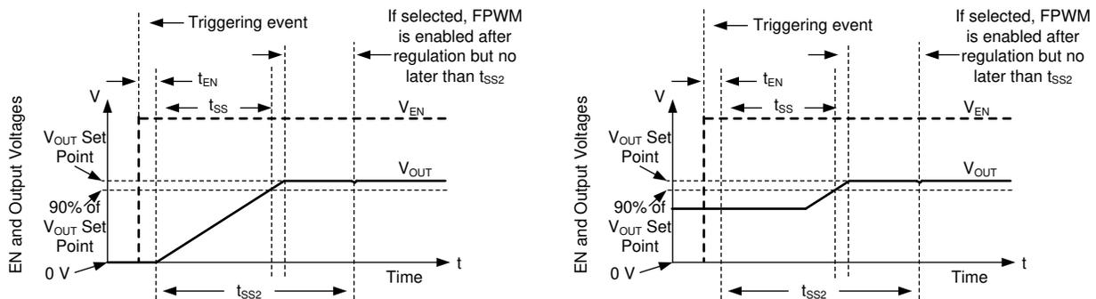
The left curves show soft start from 0 V. The right curves show soft starting behavior from a pre-biased or non-zero voltage. In either case, the output voltage reaches within 10% of the desired setpoint  $t_{SS}$  time after soft start is initiated. During soft start, FPWM and hiccup are disabled. Both hiccup and FPWM are enabled once output reaches regulation or  $t_{SS2}$ , whichever happens first.
