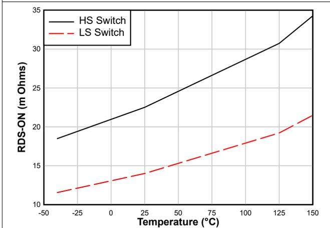
图 7-3. High-side and Low-side Switches  $R_{DS\_ON}$
