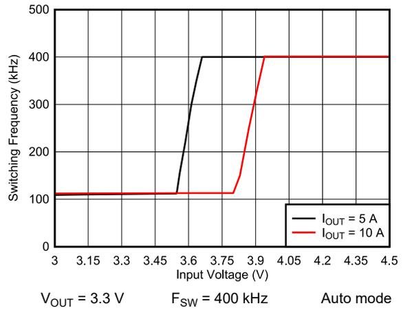
图 9-26. Frequency Dropout
