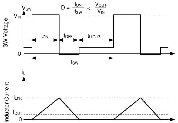
In auto mode, the low-side device is turned off once inductor current is near zero. As a result, once output current is less than half of inductor ripple in CCM, the part operates in DCM. This is equivalent to saying that diode emulation is active.
