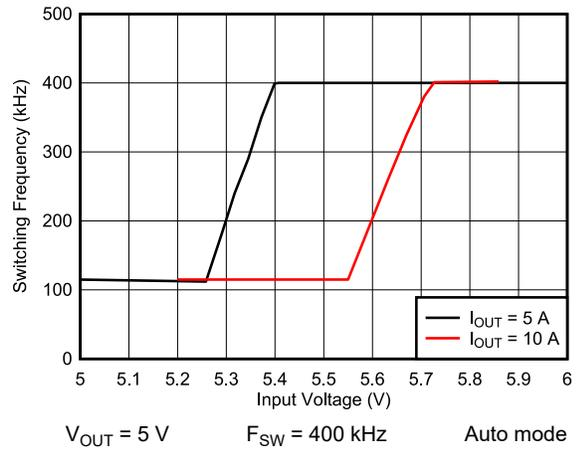
图 9-25. Frequency Dropout
