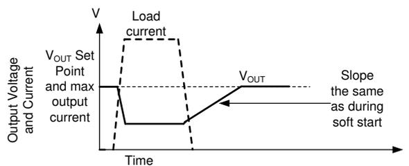
Whether output voltage falls due to high load or low input voltage, once the condition that causes output to fall below its setpoint is removed, output climbs at the same speed as during start-up. Even though hiccup does not trigger due to dropout, it can, in principal, be triggered during recovery if output voltage is below 0.4 times output the setpoint for more than 128 clock cycles during recovery.
