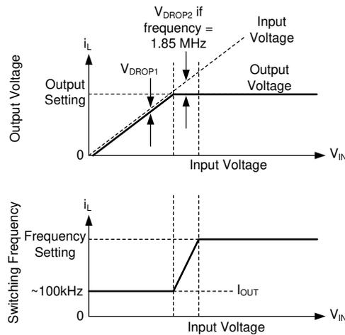
Output voltage and frequency versus input voltage: If there is little difference between input voltage and output voltage setting, the IC reduces frequency to maintain regulation. If input voltage is too low to provide the desired output voltage at approximately 110 kHz, output voltage tracks input voltage.
