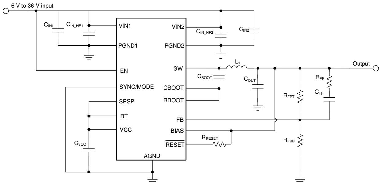
图 9-1. Example Application Circuit - 400-kHz Adjustable Output
