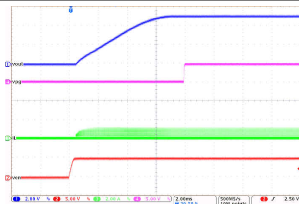
图 9-32. LM61430-Q1 Start-up with 100-mA Load
