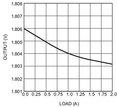
$V_{IN} = 3V$   $V_{OUT} = 1.8V$
