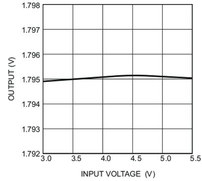
$V_{OUT} = 1.8V$   $I_{OUT} = 1000mA$
