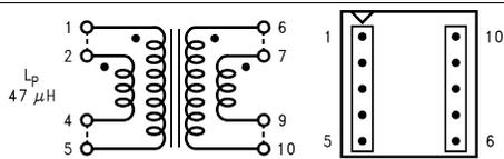
**Figure 45. Schott 26606 (Top View)**
