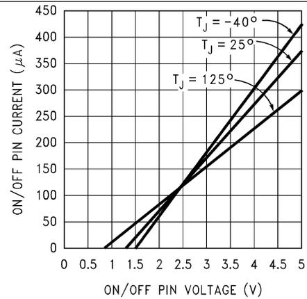
**Figure 14.  $\overline{\text{ON}}$ /Off Pin Current vs Voltage**
