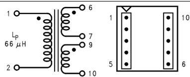
**Figure 46. Schott 67140900 (Top View)**
