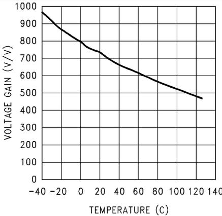
Figure 11. Error Amp Voltage Gain vs Temperature
