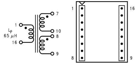
**Figure 40. Pulse PE-68414 (Surface Mount) (Top View)**
