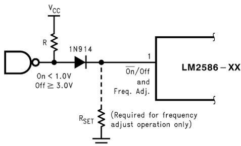
Figure 23. Shutdown Operation
