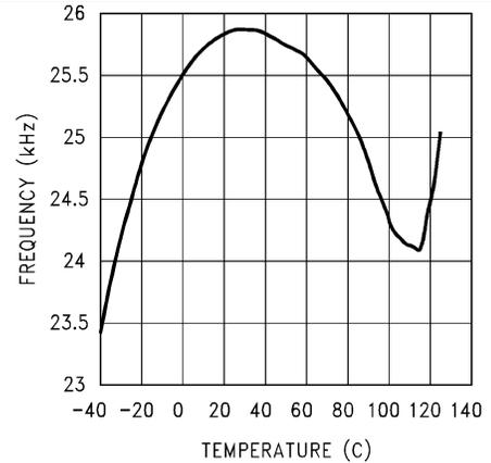
Figure 12. Short Circuit Frequency vs Temperature
