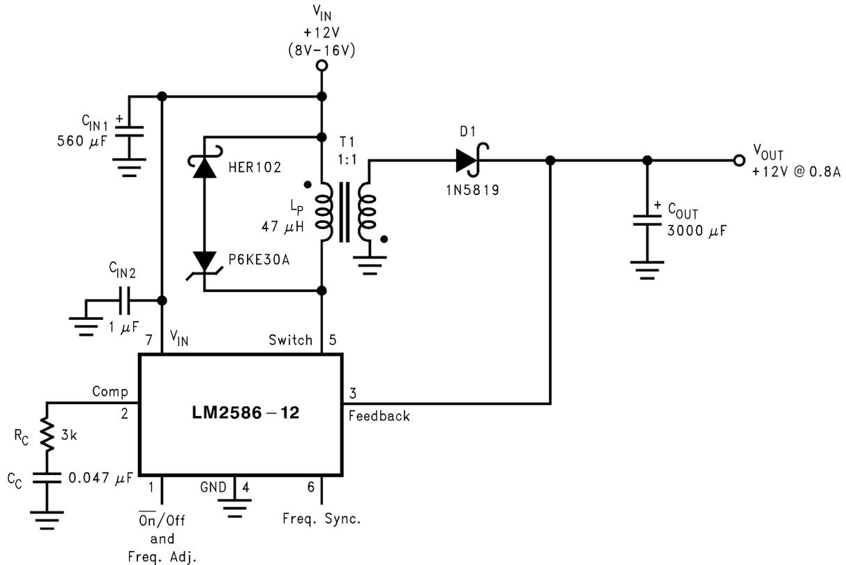
As shown in Figure 16, the LM2586 can be used as a flyback regulator by using a minimum number of external components. The switching waveforms of this regulator are shown in . Typical performance characteristics observed during the operation of this circuit are shown in .
