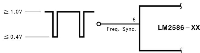
**Figure 24. Frequency Synchronization**
