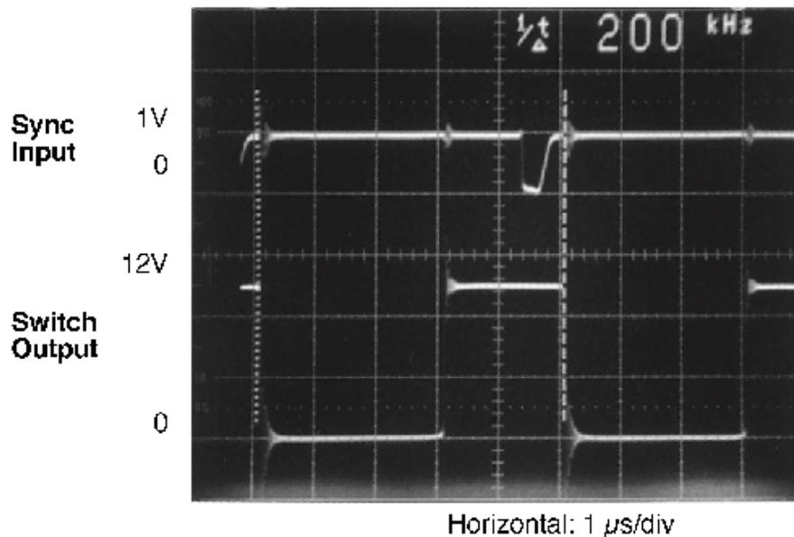
**Figure 25. Waveforms of a Synchronized 12-V Boost Regulator**
