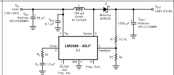
The LM2586 requires a heat sink in this application. The size of the heat sink depends on the maximum ambient temperature. To calculate the thermal resistance of the IC and the size of the heat sink needed, see [Heat Sink/Thermal Considerations](#).
