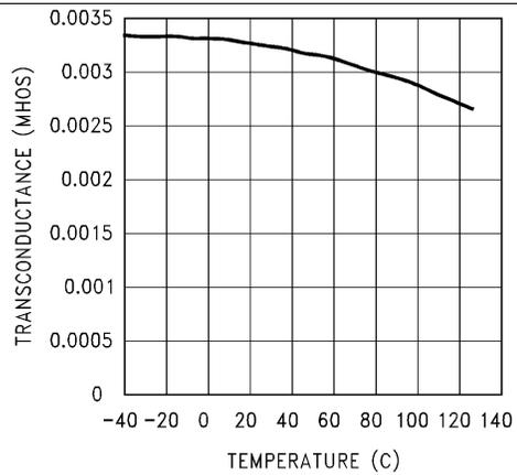
Figure 10. Error Amp Transconductance vs Temperature
