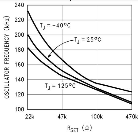
**Figure 15. Oscillator Frequency vs Resistance**
