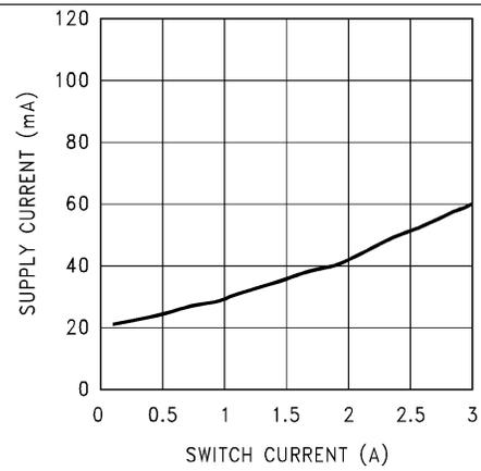
Figure 4. Supply Current vs Switch Current
