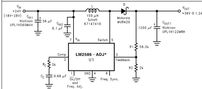
The LM2586 requires a heat sink in this application. The size of the heat sink depends on the maximum ambient temperature. To calculate the thermal resistance of the IC and the size of the heat sink needed, see [Heat Sink/Thermal Considerations](#).
