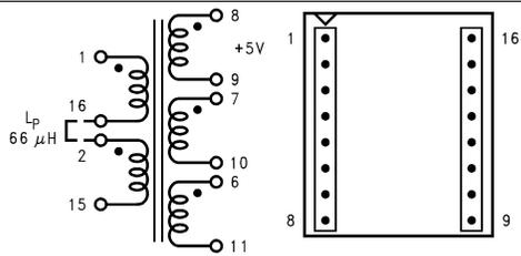
**Figure 41. Pulse PE-68413 (Surface Mount) (Top View)**
