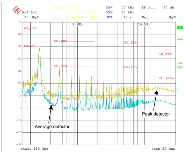
图 8-14. CISPR 25 Class 5 Conducted EMI Plot
