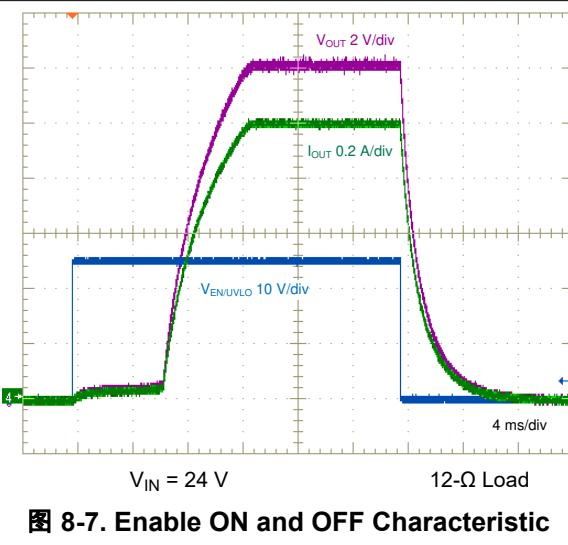
图 8-7. Enable ON and OFF Characteristic
