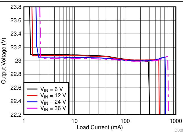
图 8-20. Load Regulation (Log Scale)
