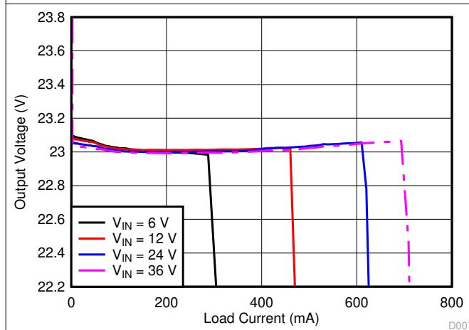
图 8-19. Load Regulation (Linear Scale)
