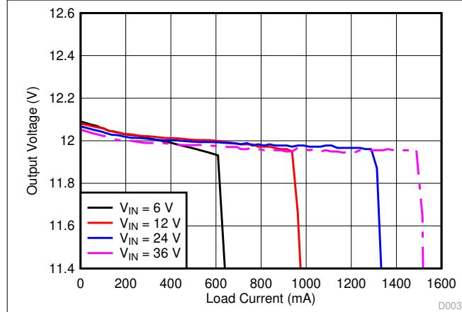
图 8-4. Load Regulation (Linear Scale)
