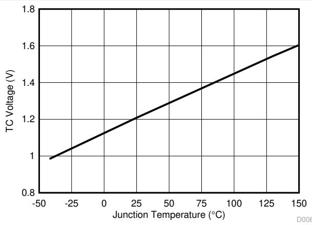
**图 6-9. TC Voltage versus Temperature**
