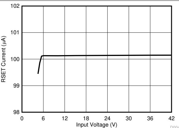
**图 6-7. RSET Current versus Input Voltage**
