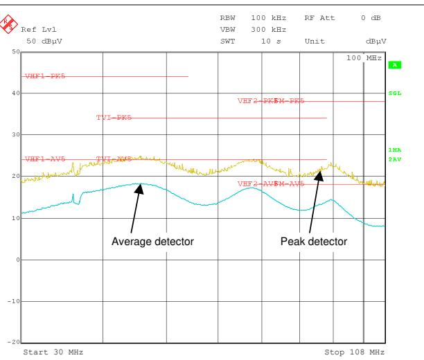
图 8-15. CISPR 25 Class 5 Conducted EMI Plot
