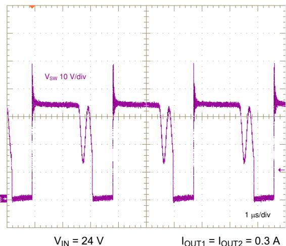
图 8-23. Switch Voltage, Medium Load
