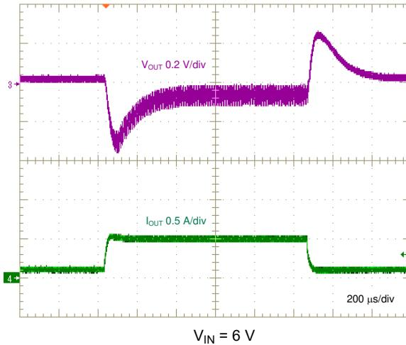
图 8-13. Load Transient, 0.1 A to 0.5 A, 0.1 A/μs
