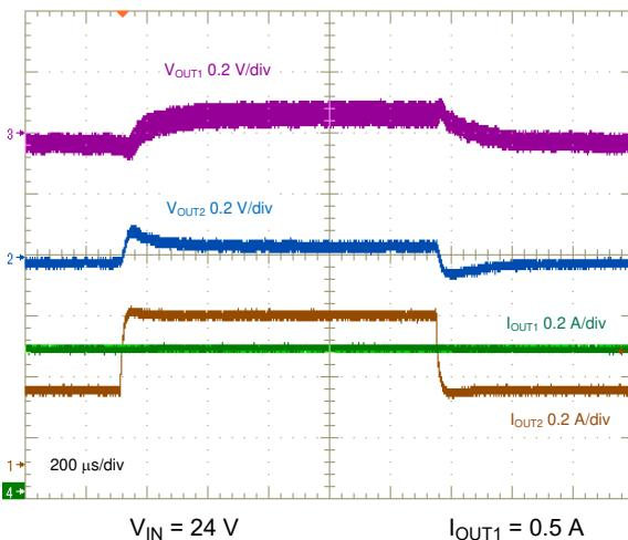
图 8-26. Negative Output Load Transient, 0.25 A to 0.5 A
