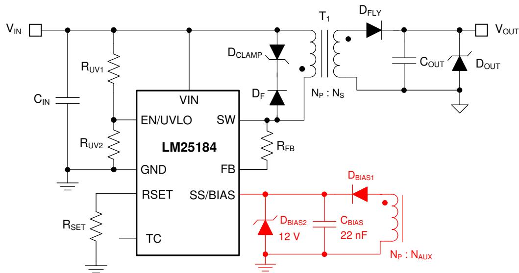
**图 7-4. External Bias Supply Using Transformer Auxiliary Winding**
