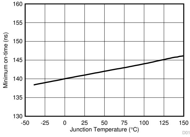
**图 6-12. Minimum Switch On-Time versus Temperature**
