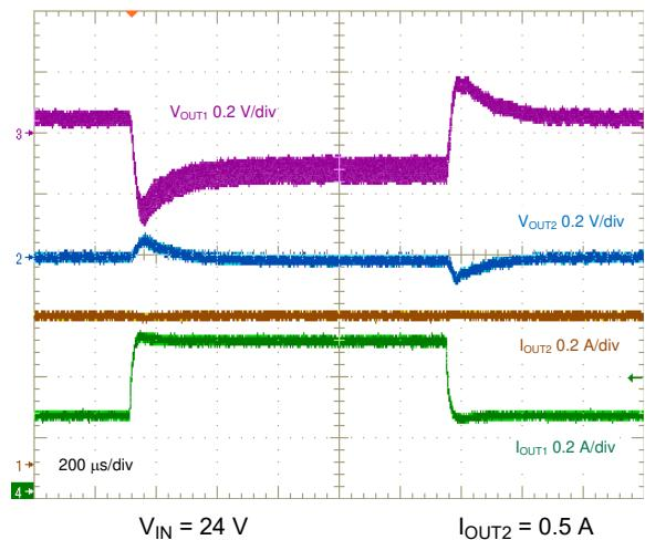
图 8-25. Positive Output Load Transient, 0.25 A to 0.5 A
