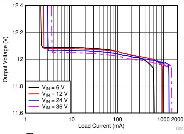
图 8-5. Load Regulation (Log Scale)
