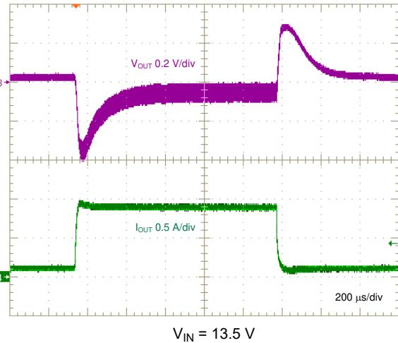
图 8-12. Load Transient, 0.1 A to 1 A, 0.1 A/μs
