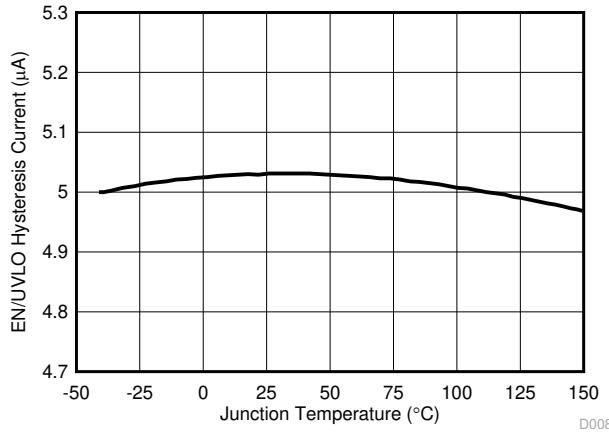
**图 6-11. EN/UVLO Hysteresis Current versus Temperature**
