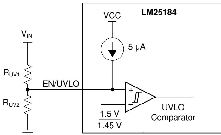
**图 7-3. Programmable Input Voltage UVLO With Hysteresis**
