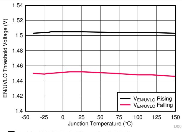
**图 6-10. EN/UVLO Threshold Voltages versus Temperature**
