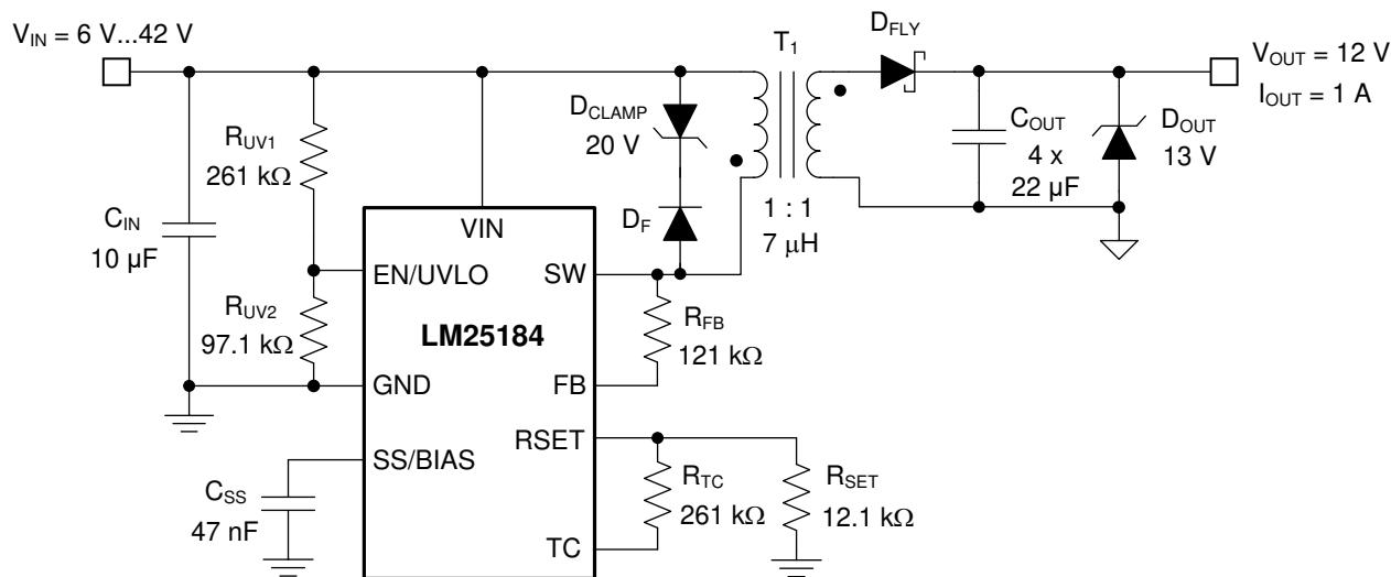
**图 8-1. Schematic for Design 1 With  $V_{IN(nom)} = 24$  V,  $V_{OUT} = 12$  V,  $I_{OUT} = 1$  A**
