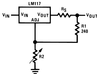
图 8-1. Regulator With Line Resistance in Output Lead
