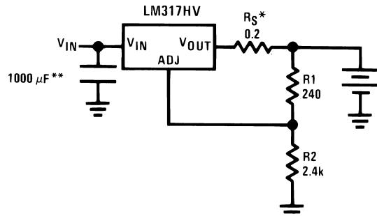
$$*R_S \text{—sets output impedance of charger } Z_{\text{OUT}} = R_S \left( 1 + \frac{R_2}{R_1} \right)$$
