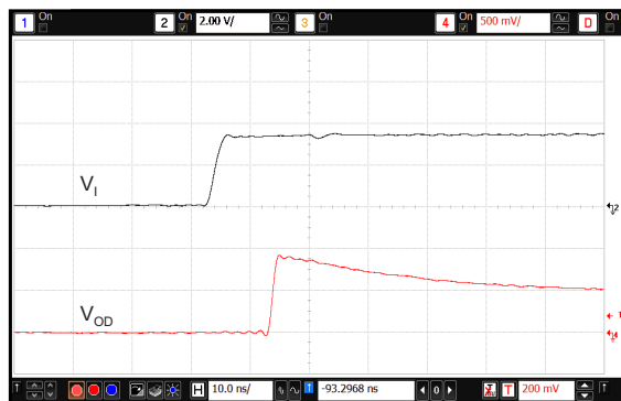
Figure 15. Distortion Correction Scheme Calibration Time ( t_{CALIB} )
