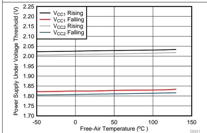
Figure 5. Power Supply Undervoltage Threshold vs Free-Air Temperature
