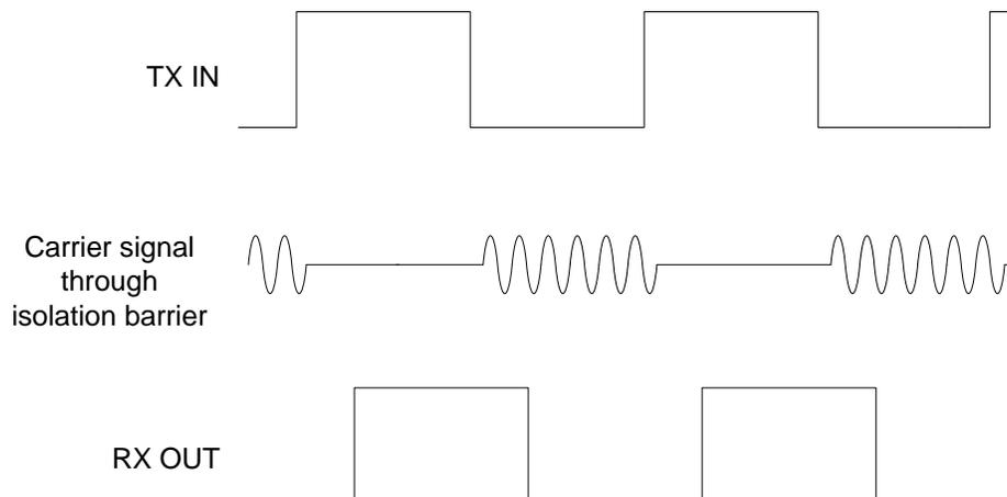
**Figure 11. On-Off Keying (OOK) Based Modulation Scheme**
