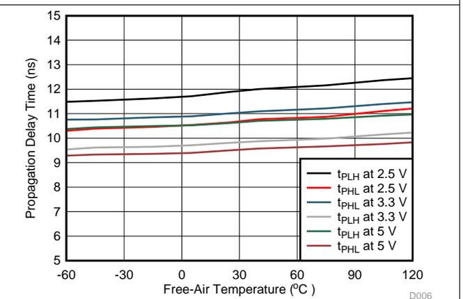
Figure 6. Propagation Delay Time vs Free-Air Temperature
