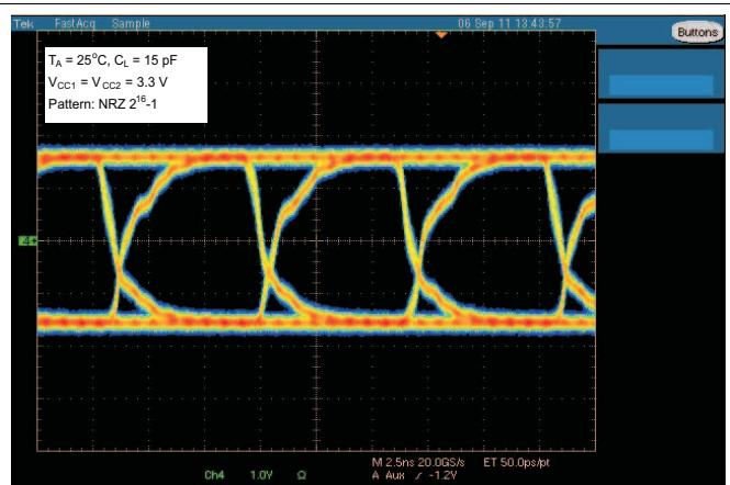
图 20. Typical Eye Diagram at 150 Mbps,
