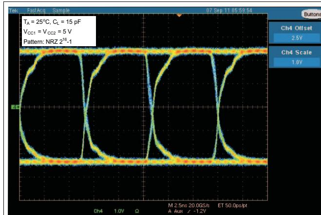
图 19. Typical Eye Diagram at 150 Mbps,
