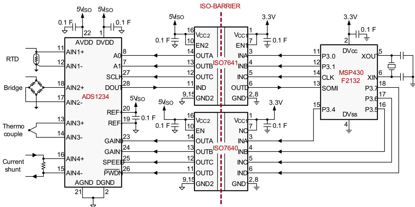
图 16. Isolated Data Acquisition System for Process Control
