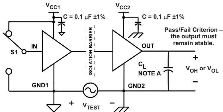
A.  $C_L = 15 \text{ pF}$  and includes instrumentation and fixture capacitance within  $\pm 20\%$ .
