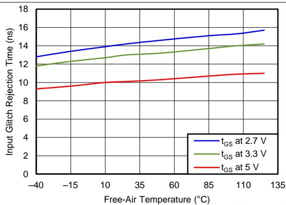
**Figure 8. Input Glitch Suppression Time vs Free-Air Temperature**
