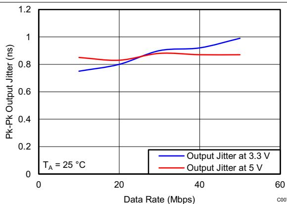
**Figure 7. Output Jitter vs Data Rate**
