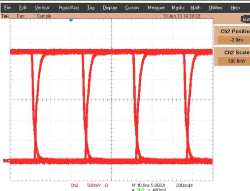
**Figure 11. Eye Diagram at 40 Mbps, 2.7V at 25°C**
