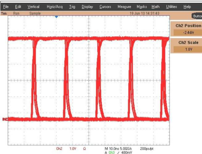
**Figure 9. Eye Diagram at 50 Mbps, 5V at 25°C**
