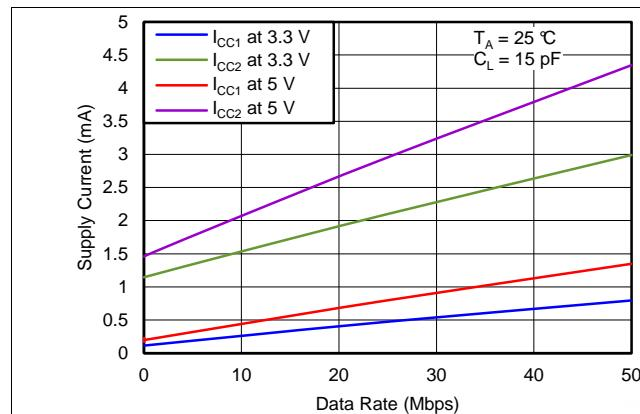
Figure 1. Supply Current Per Channel vs Data Rate
