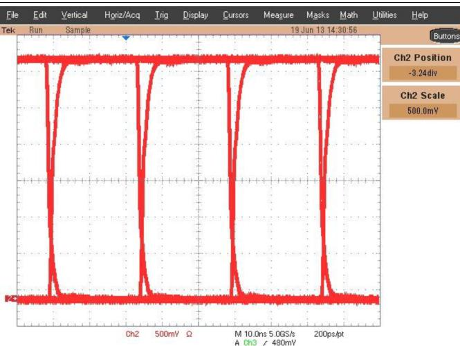
**Figure 10. Eye Diagram at 40 Mbps, 3.3V at 25°C**
