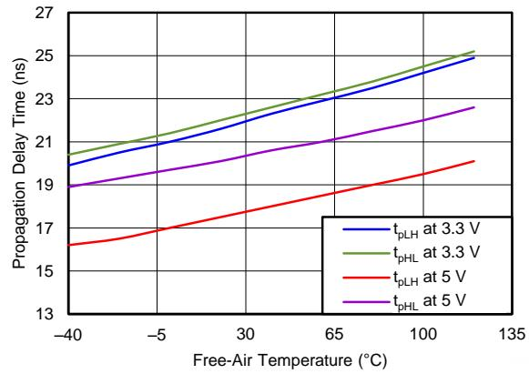
Figure 6. Propagation Delay Time vs Free-Air Temperature
