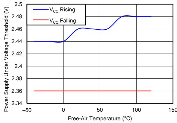
Figure 5.  $V_{CC1}$  and  $V_{CC2}$  Undervoltage Threshold vs Free-Air Temperature
