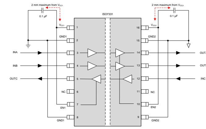
Figure 22. Typical ISO7331-Q1 Circuit Hook-up
