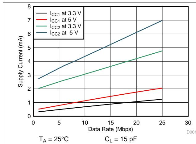
**Figure 1. ISO7330-Q1 Supply Current vs Data Rate (With 15-pF Load)**
