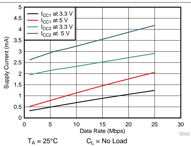
**Figure 2. ISO7330-Q1 Supply Current vs Data Rate (With No Load)**
