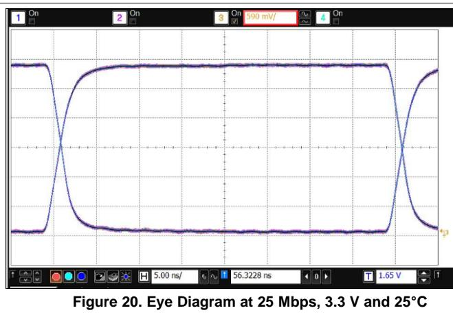
Figure 20. Eye Diagram at 25 Mbps, 3.3 V and 25°C
