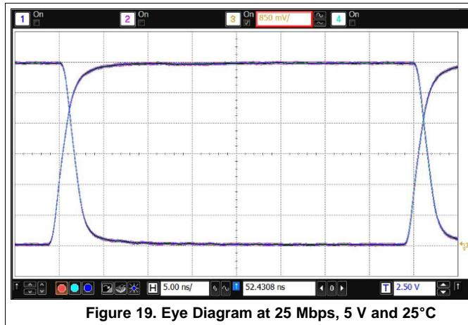
Figure 19. Eye Diagram at 25 Mbps, 5 V and 25°C
