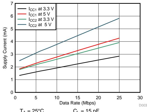
**Figure 3. ISO7331-Q1 Supply Current vs Data Rate (With 15-pF Load)**
