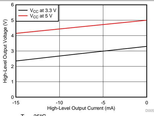
**Figure 5. High-Level Output Voltage vs High-level Output Current**
