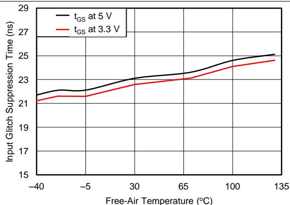
**Figure 7. Input Glitch Suppression Time vs Free-Air Temperature**
