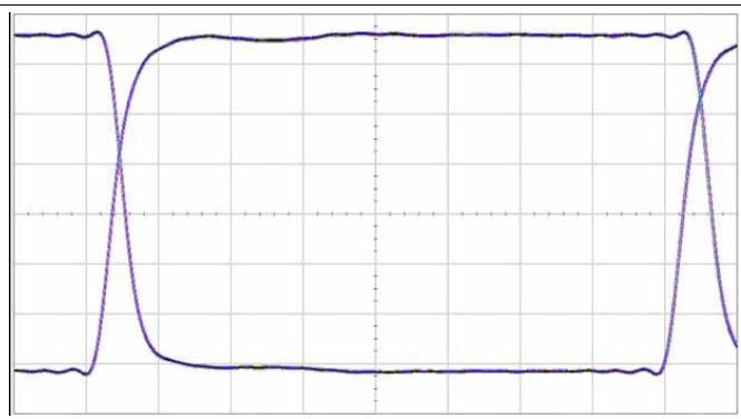
Figure 18. Eye Diagram at 25 Mbps, 3.3 V and 25°C
