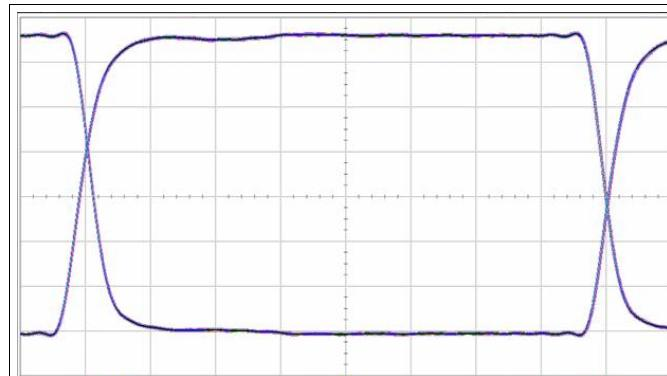
Figure 17. Eye Diagram at 25 Mbps, 5 V and 25°C
