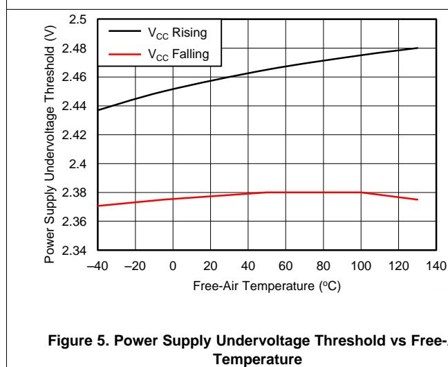
Figure 5. Power Supply Undervoltage Threshold vs Free-Air Temperature
