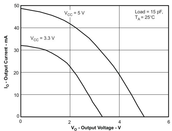
图 4-6. High-Level Output Current vs High-Level Output Voltage
