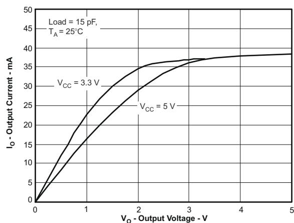
图 4-7. Low-Level Output Current vs Low-Level Output Voltage
