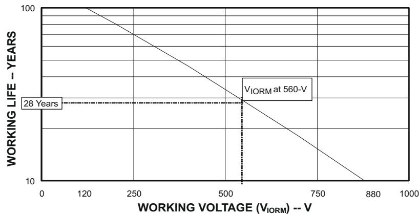
图 7-3. Time Dependent Dielectric Breakdown Testing Results
