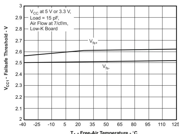
图 4-5.  $V_{CC1}$  Failsafe Threshold vs Free-Air Temperature
