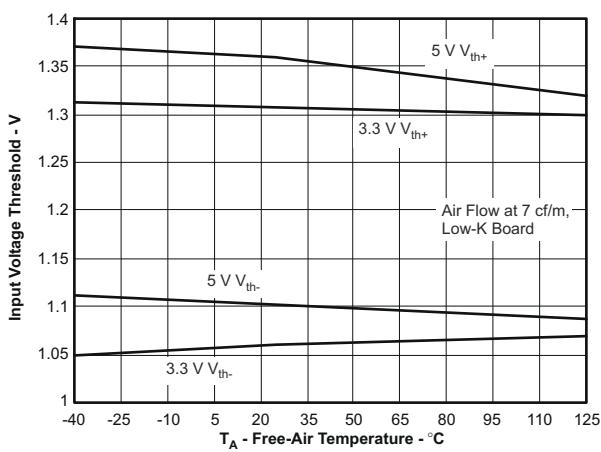
图 4-4. Input Threshold Voltage vs Free-Air Temperature
