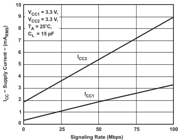
图 6-1. RMS Supply Current Versus Signaling Rate
