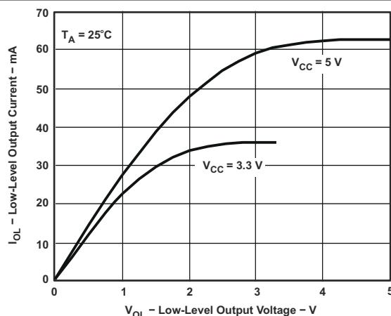
图 6-8. Low-Level Output Current Versus Low-Level Output Voltage
