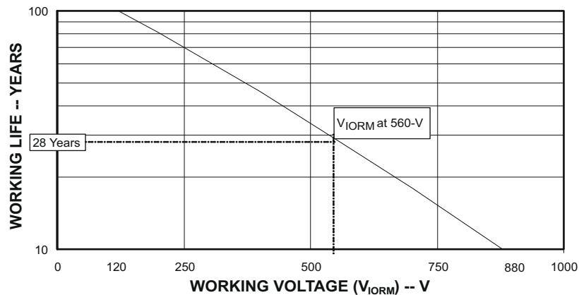
图 6-9. Time Dependent Dielectric Breakdown Testing Results
