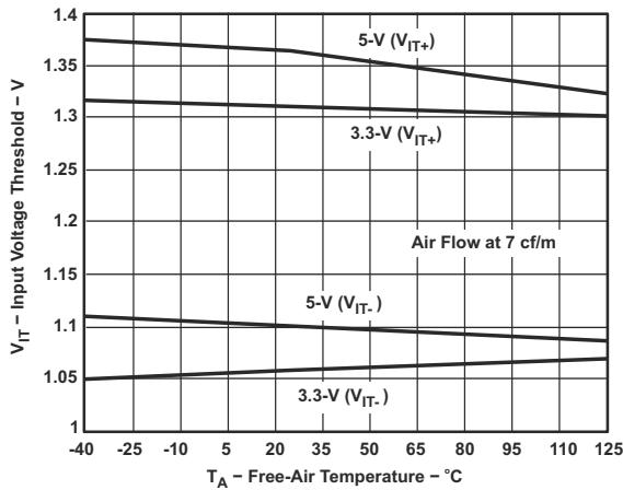
图 6-5. Input Threshold Voltage Versus Free-Air Temperature
