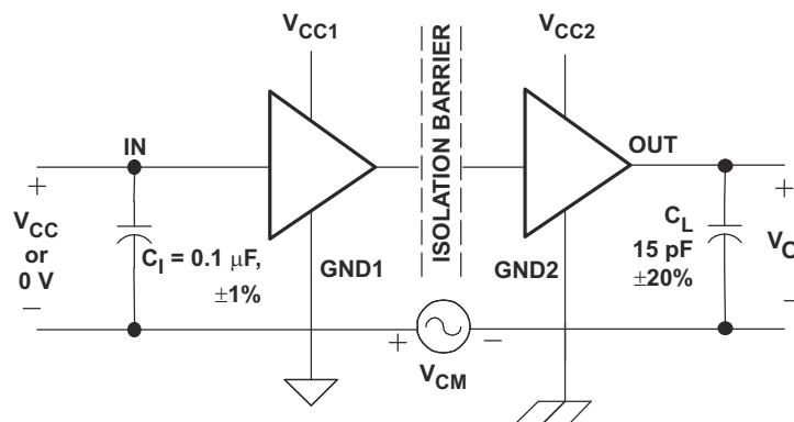
图 7-5. Common-Mode Transient-Immunity Test Circuit and Voltage Waveform
