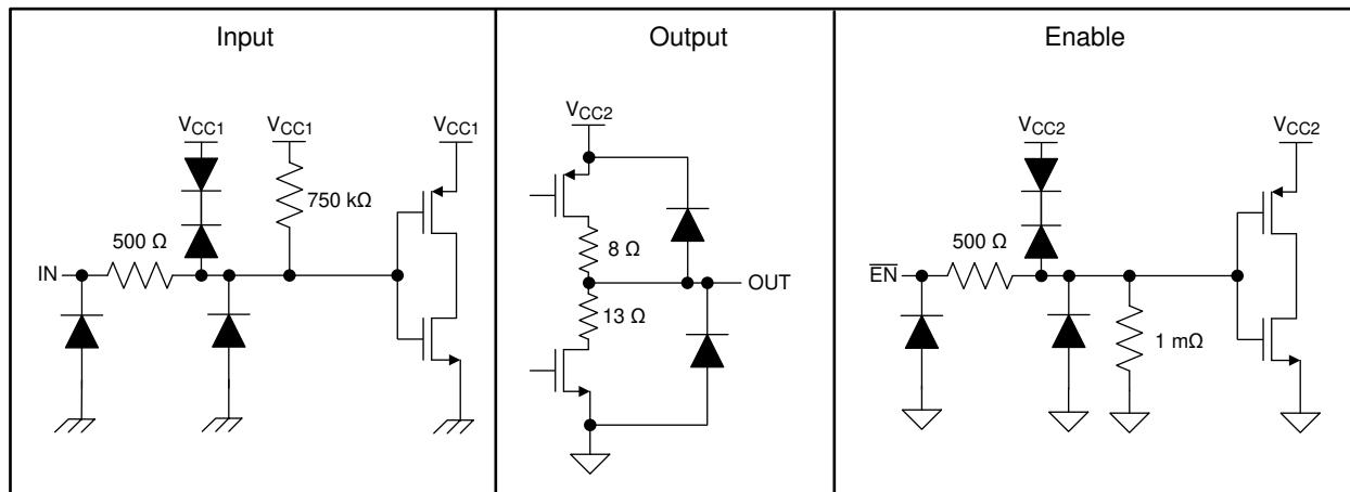
图 8-1. Equivalent Input and Output Schematic Diagrams
