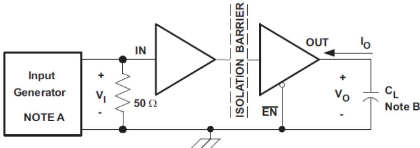
图 7-1. Switching Characteristic Test Circuit and Voltage Waveforms
