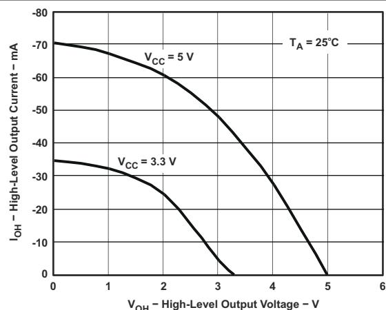
图 6-7. High-Level Output Current Versus High-Level Output Voltage
