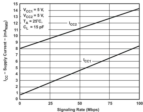
图 6-2. RMS Supply Current Versus Signaling Rate
