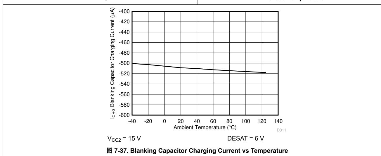
图 7-37. Blanking Capacitor Charging Current vs Temperature
