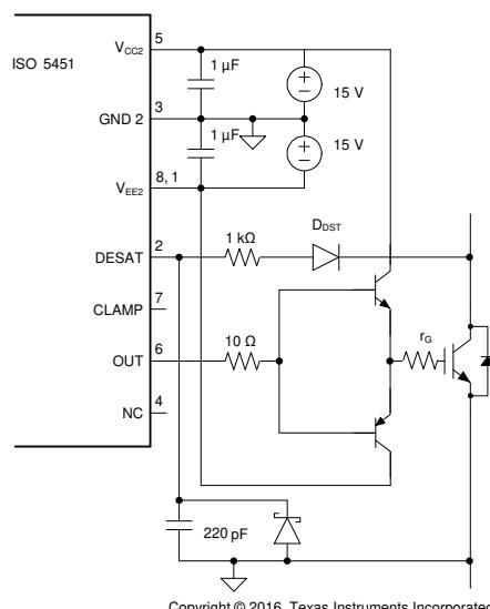
图 10-10. Current Buffer for Increased Drive Current
