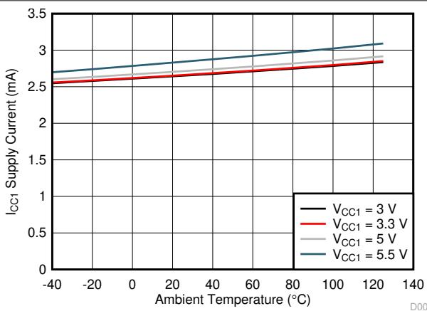
图 7-16. I<sub>CC1</sub> Supply Current vs Temperature
