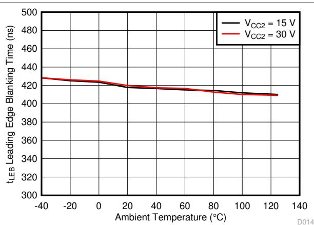
图 7-29. Leading Edge Blanking Time With Temperature
