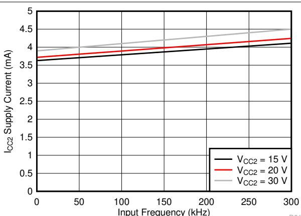
图 7-20. I<sub>CC2</sub> Supply Current vs Input Frequency
