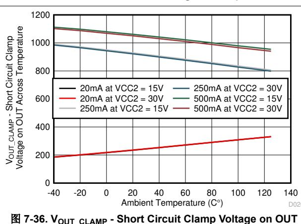
图 7-36.  $V_{OUT\text{ Clamp}}$  - Short Circuit Clamp Voltage on OUT Across Temperature
