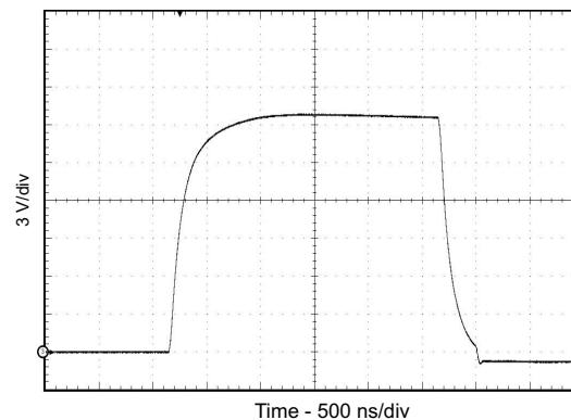
$C_L = 10 \text{ nF}$        $R_G = 10 \Omega$
