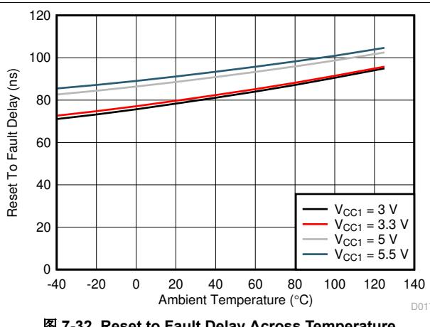
图 7-32. Reset to Fault Delay Across Temperature
