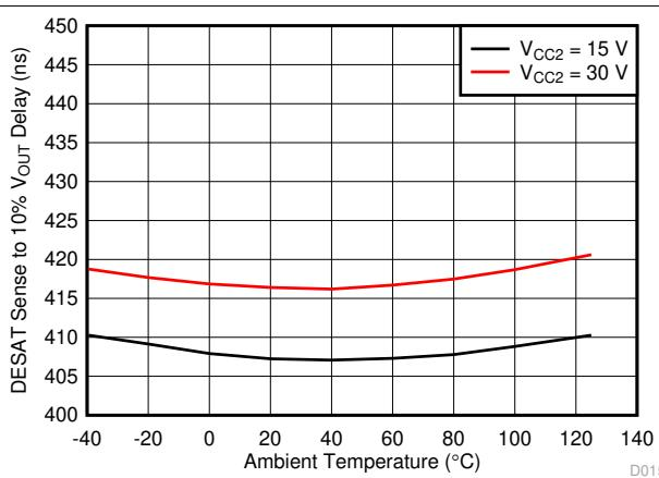
图 7-30. DESAT Sense to  $V_{OUT}$  10% Delay vs Temperature
