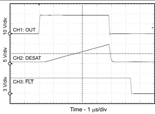
图 7-15. Output Transient Waveform DESAT and FLT
