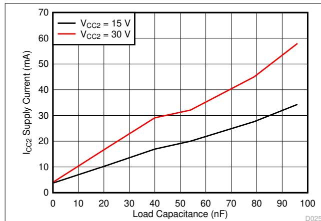
$R_G = 10\text{ }\Omega$ , 20kHz
