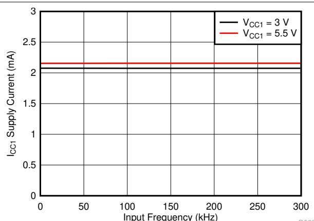
图 7-19. I<sub>CC1</sub> Supply Current vs Input Frequency
