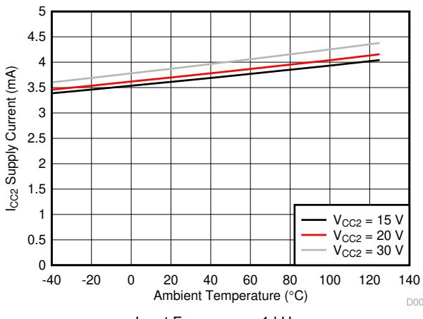
图 7-18. I<sub>CC2</sub> Supply Current vs Temperature
