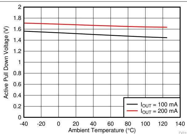
图 7-34. Active Pull Down Voltage vs Temperature
