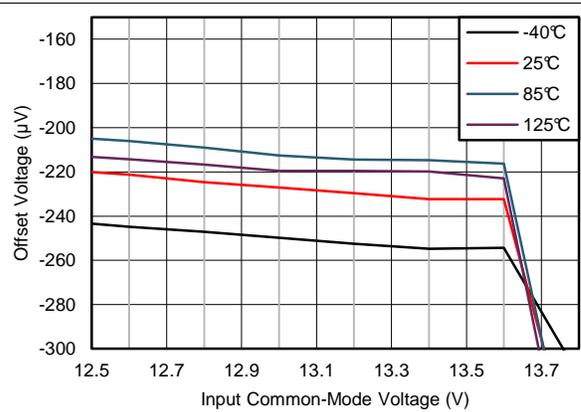
图 34. Offset Voltage vs Positive Common-Mode Voltage
