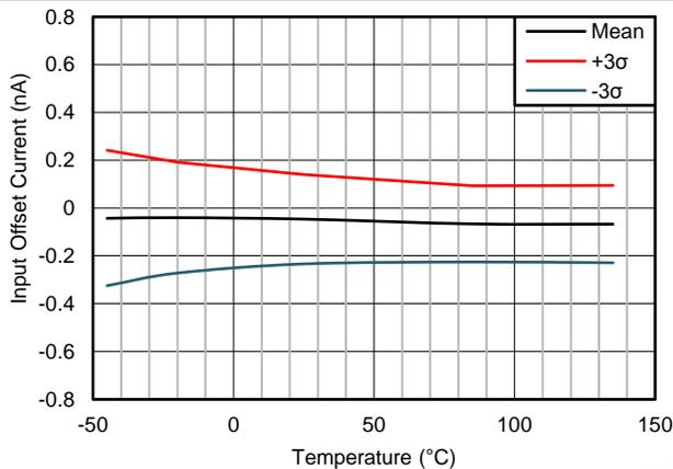
图 11. Input Offset Current vs Temperature
