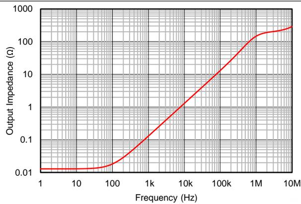
图 45. Closed-Loop Output Impedance
