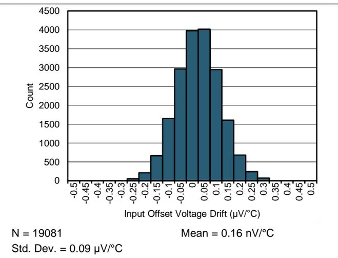
图 2. Typical Distribution of Input Offset Voltage Drift
