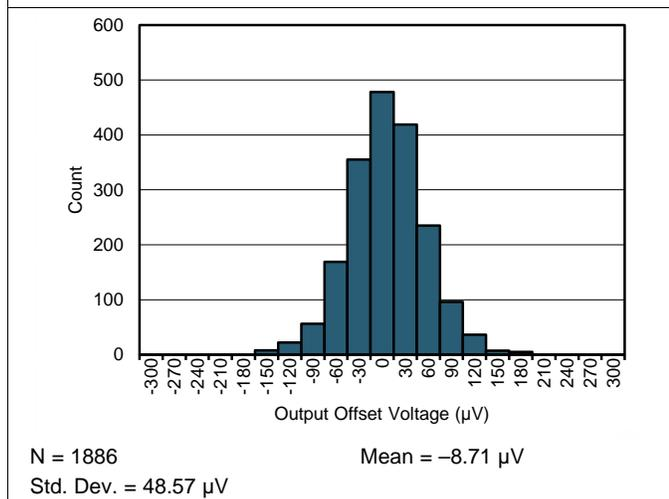
图 3. Typical Distribution of Output Offset Voltage
