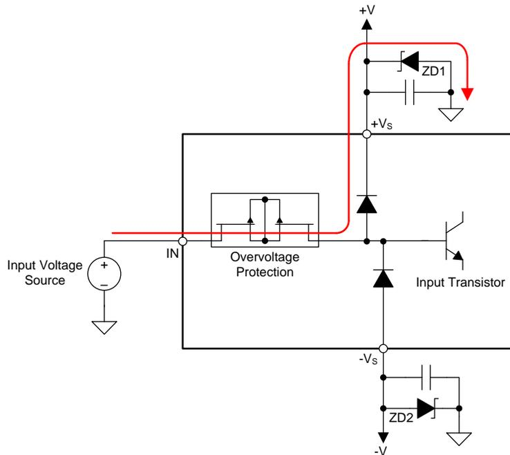
图 59. Input Current Path During an Overvoltage Condition
