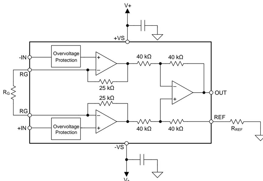
**图 61. Parasitic Resistance Shown at the Reference Terminal**
