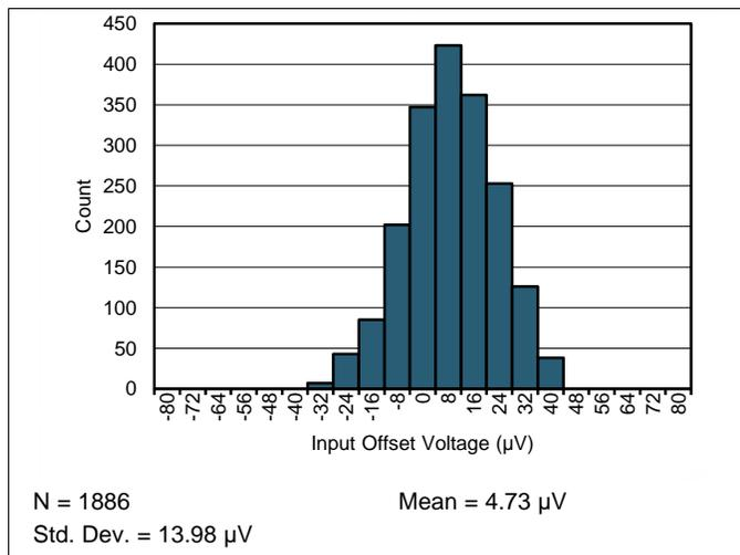
图 1. Typical Distribution of Input Offset Voltage
