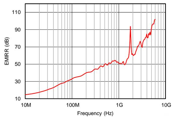
图 46. Differential-Mode EMI Rejection Ratio
