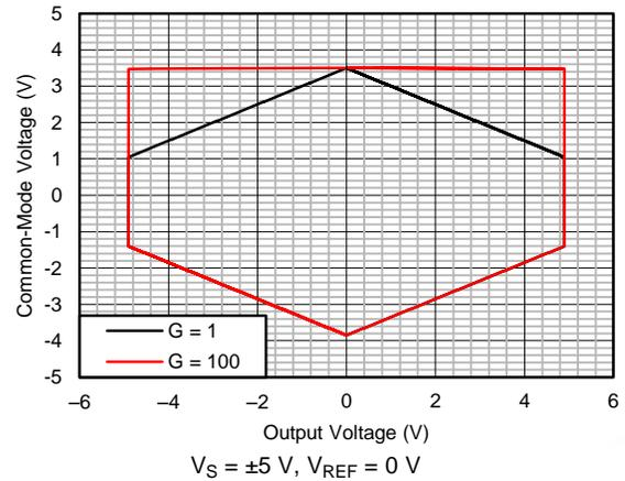
图 50. Input Common-Mode Voltage vs Output Voltage
