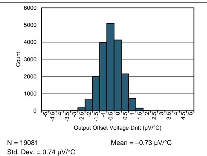
图 4. Typical Distribution of Output Offset Voltage Drift
