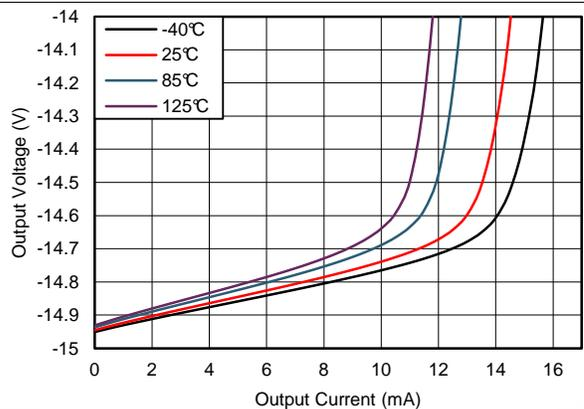
图 36. Negative Output Voltage Swing vs Output Current
