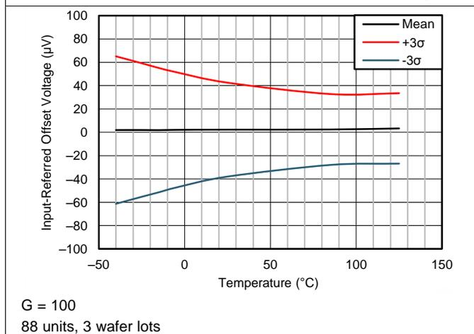
图 5. Input-Referred Offset Voltage vs Temperature
