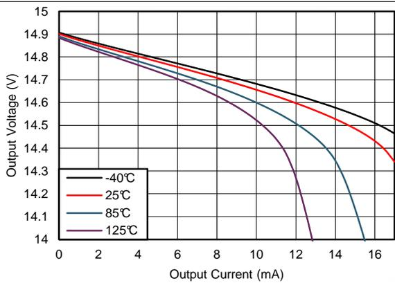
图 35. Positive Output Voltage Swing vs Output Current
