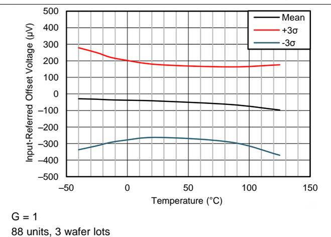
图 6. Input-Referred Offset Voltage vs Temperature
