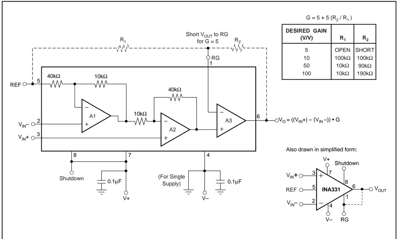
FIGURE 1. Basic Connections.
