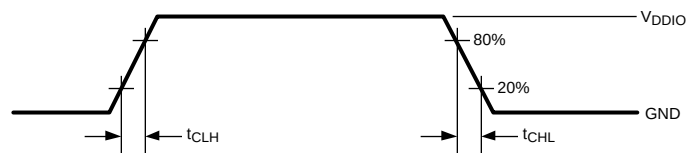
Figure 3. LVCMOS Transition Times
