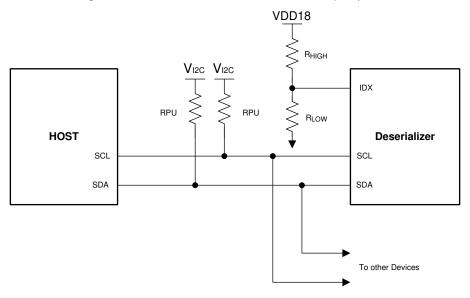
图 7-19. Serial Control Bus Connection
