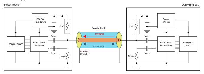
图 8-1. Power-over-Coax (PoC) System Diagram
