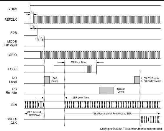
图 9-2. Power-Up Sequencing With Synchronous Clocking Mode
