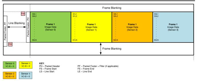
\*Blanking intervals do not provide accurate synchronization timing
