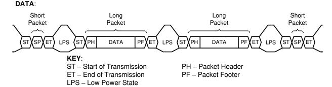
图 7-7. CSI-2 Protocol Layer With Short and Long Packets
