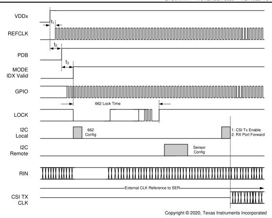
图 9-3. Power-Up Sequencing With Non-Synchronous Clocking Mode
