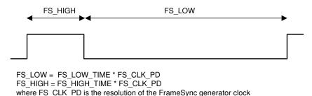
图 7-15. Internal FrameSync Signal
