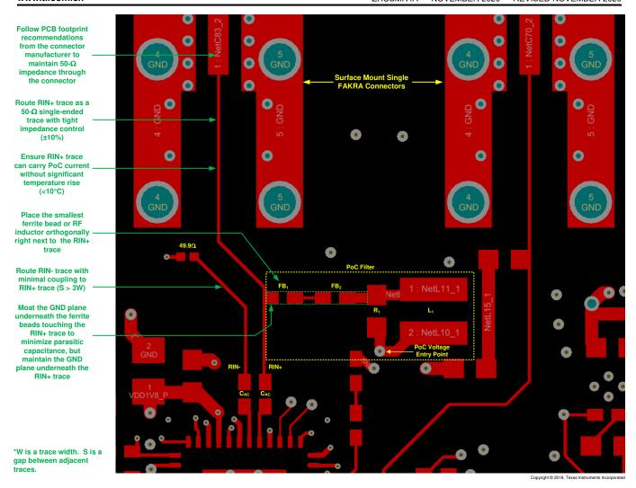
图 10-2. Example Routing of FPD-Link III Traces to a Single Mini-Fakra Connector and PoC Components
