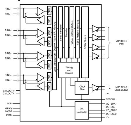
图 7-1. Functional Block Diagram
