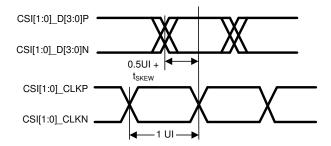
图 6-5. Clock and Data Timing in HS Transmission
