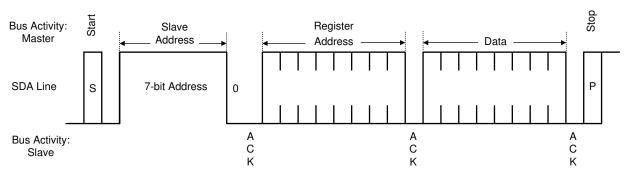
图 7-22. Serial Control Bus — WRITE
