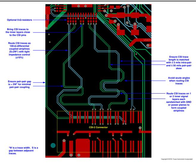
图 10-3. Example Routing of CSI-2 Traces
