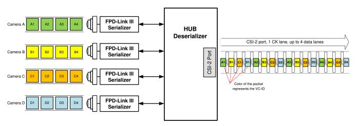
图 7-12. Four Sensor Data onto CSI-2 With Virtual Channels (VC-ID)
