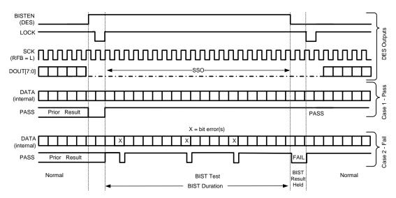
Figure 29. BIST Timing Diagram
