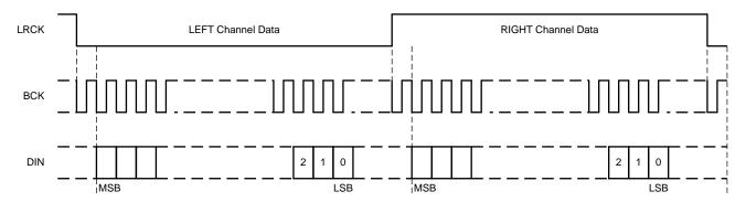
Figure 16. Stereo I<sup>2</sup>S Format
