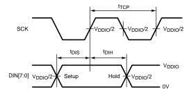
Figure 10. Serializer Setup/Hold Times
