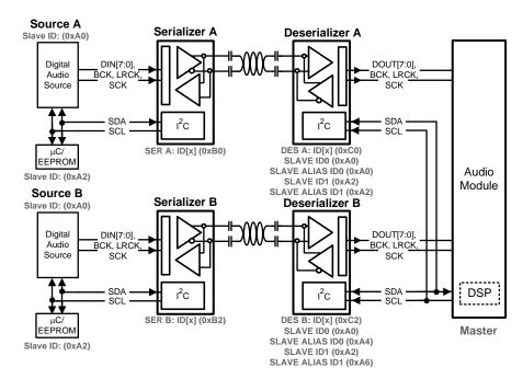
Figure 26. Multiple Device Addressing
