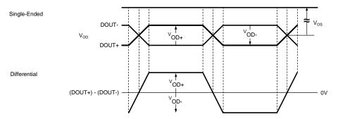
Figure 8. Serializer VOD and Differential Diagram
