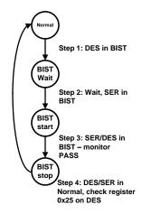
Figure 28. BIST System Flow Diagram
