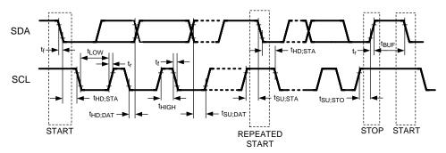
Figure 4. Bidirectional Control Bus Timing
