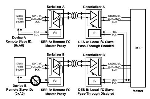
Figure 25. I<sup>2</sup>C Pass-Through
