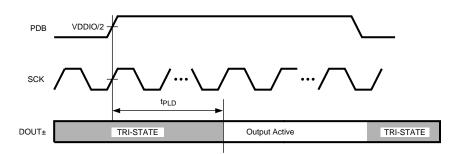
Figure 11. Serializer PLL Lock Time
