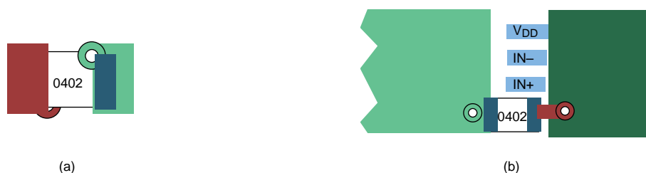
Figure 21. Typical Decoupling Capacitor Layouts
