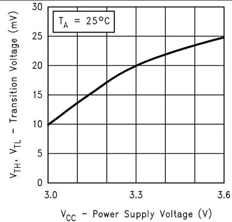
Figure 4. Differential Transition Voltage vs Power Supply Voltage
