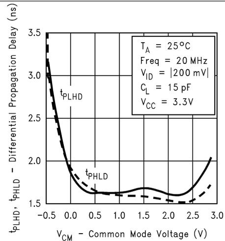
Figure 8. Differential Propagation Delay vs Common-Mode Voltage
