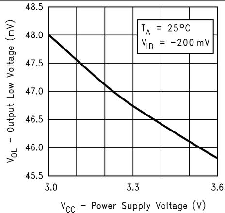
Figure 2. Output Low Voltage vs Power Supply Voltage
