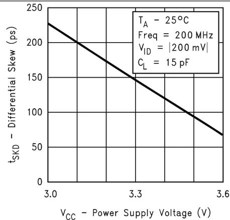
Figure 10. Differential Skew vs Power Supply Voltage
