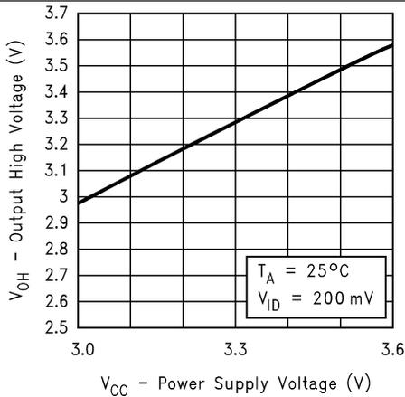
Figure 1. Output High Voltage vs Power Supply Voltage
