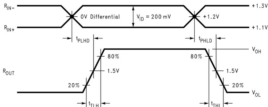
Figure 16. Receiver Propagation Delay and Transition Time Waveforms
